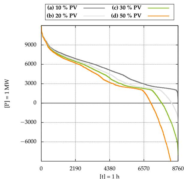
**Figure 3.** Ordered residual load profile (region) of the supply system over one year for different PV expansion stages (a)–(d).
