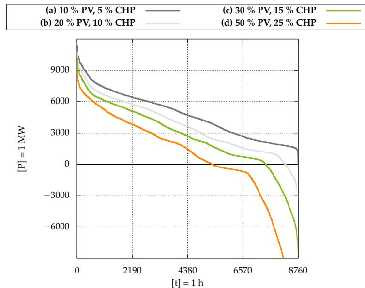
**Figure 10.** Ordered residual load profile (region) of the supply system over one year for different PV and CHP expansion stages (a)–(d).
