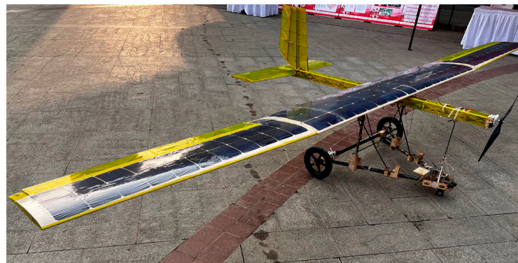
Figure 7. An overall configuration of solar-powered UAV constructed by Guo et al. [45].
