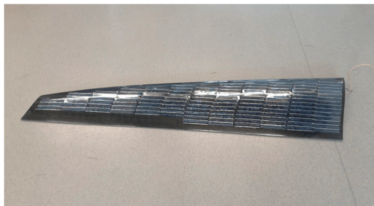
Figure 9. Ultra-light wings with embedded micro-texturized solar cells [64].
