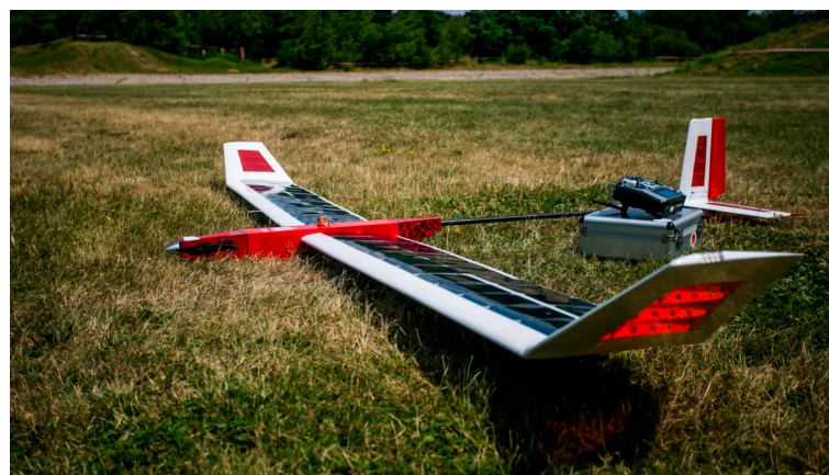
Figure 6. An overall configuration of solar-powered UAV constructed [43].
