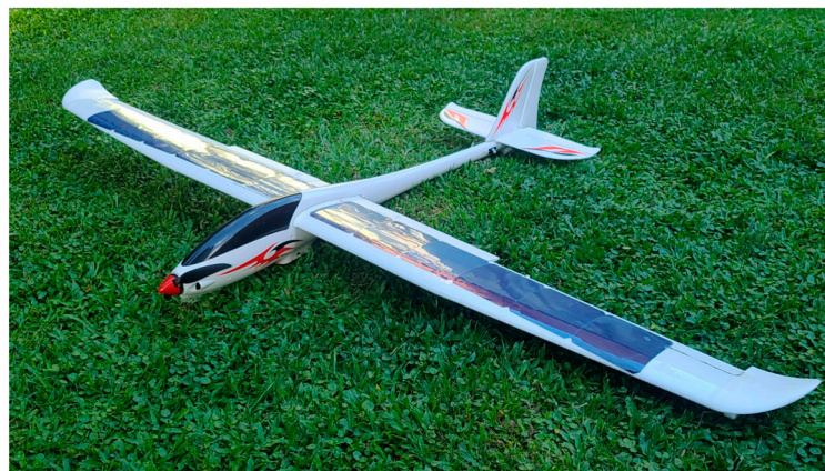
Figure 10. The solar-powered UAV developed by Chu et al. [66].
