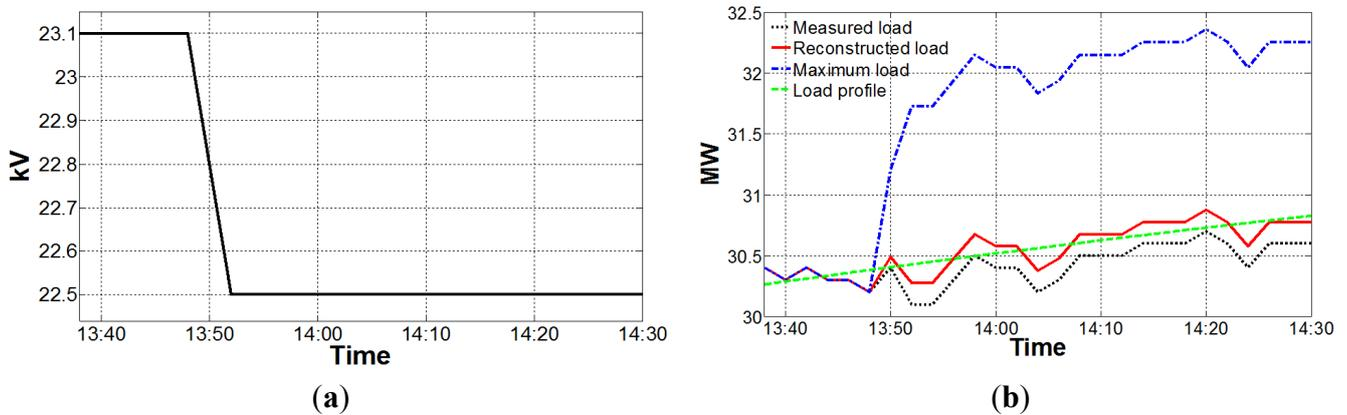
In the case of the 705th transformer bank, the inception time was 13:46 and its actual voltage reduction was about 1.75%, dropping from 22.9 kV to 22.5 kV, as shown in Figure 4a. In this case, the objective function of Equation (6) reaches its minimum value when  $p_{C705} = 1.34$ ,  $a_{2_{705}} = -0.00049$ ,  $a_{1_{705}} = 0.02345$ , and  $a_{0_{705}} = 37.7200$ .
