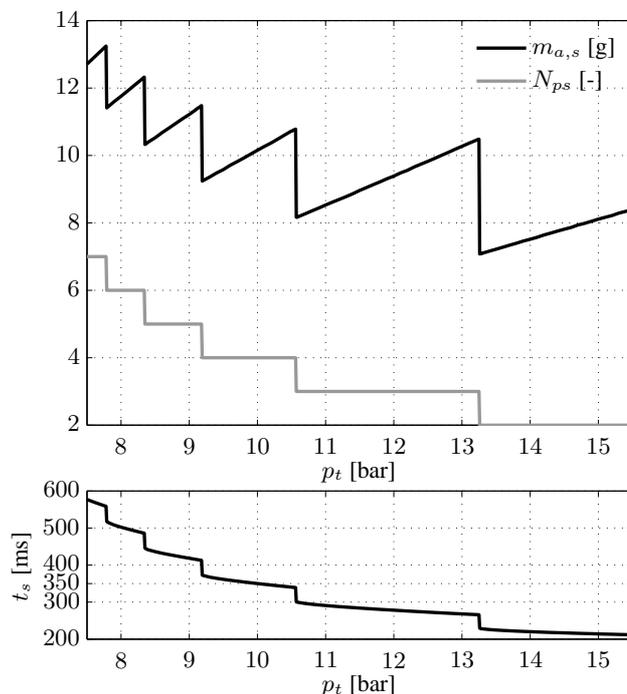
The start time is also a piecewise continuous function of the tank pressure. However, it strictly decreases as the tank pressure increases. For tank pressures lower than 10 bar, the start lasts longer than 350 ms and thus does not fulfill the performance goal. However, a start is still possible.
