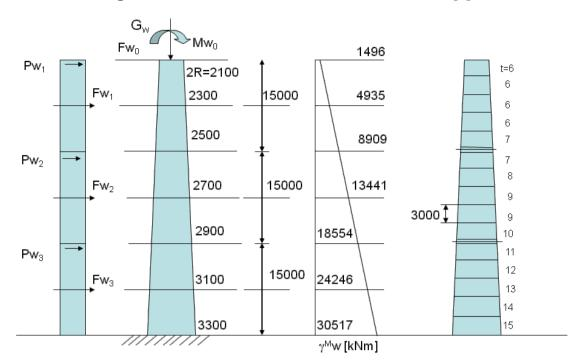
Figure 3. The 45 m wind turbine tower model used in [8].
