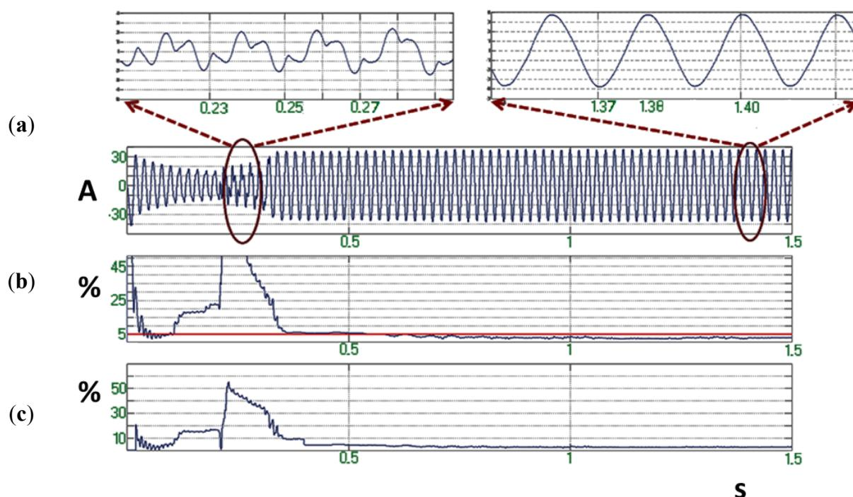
**Figure 6.** (a) Grid's current  $I_G$ ; (b) Grid's current THD; (c) Grid's current 3rd harmonic component in the second case.
