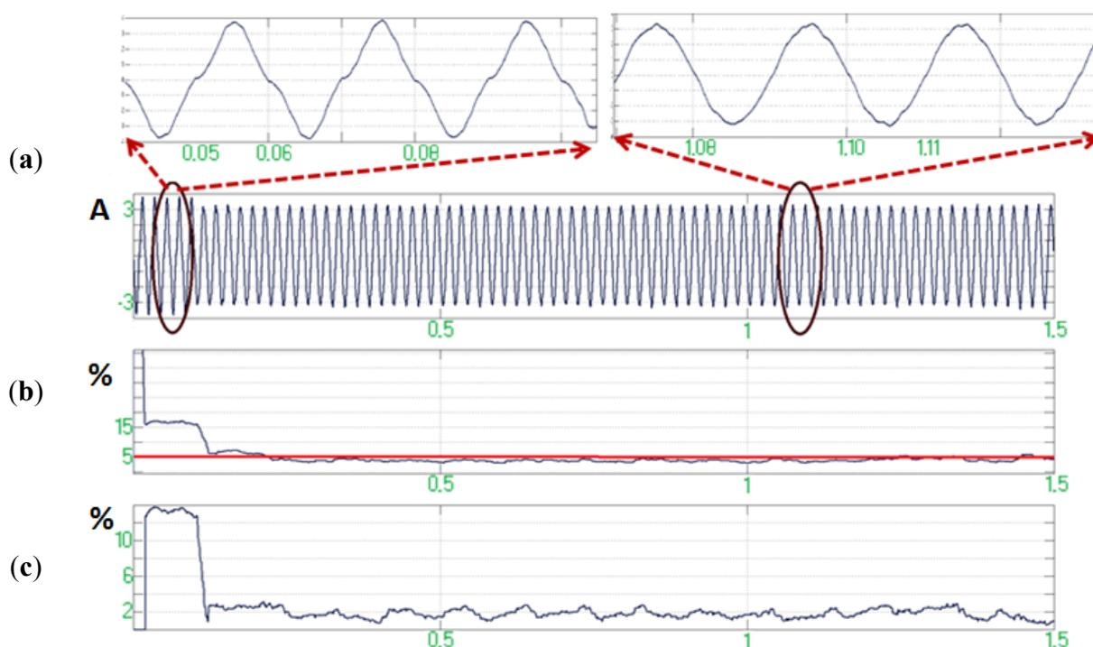
**Figure 5.** (a) Grid's current  $I_G$ ; (b) Grid's current THD; (c) Grid's current 3rd harmonic component in the first case.
