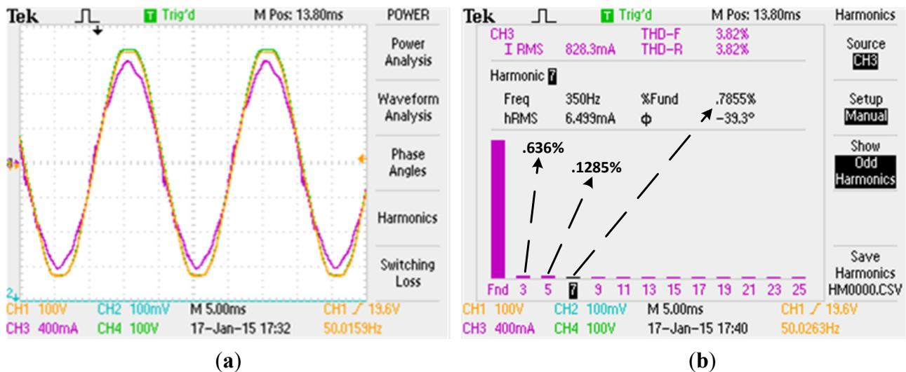
**Figure 12.** (a) Grid's voltage and current waveforms after compensation of 3rd, 5th and 7th harmonics; (b) Grid's current harmonic spectrum after compensation of 3rd, 5th and 7th harmonics.
