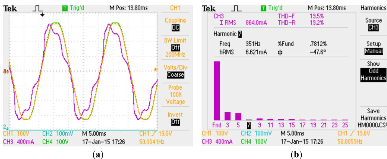
**Figure 11.** (a) Grid's voltage and current waveforms after compensation of 7th harmonic; (b) Grid's current harmonic spectrum after compensation of 7th harmonic. 7th harmonic is shown.
