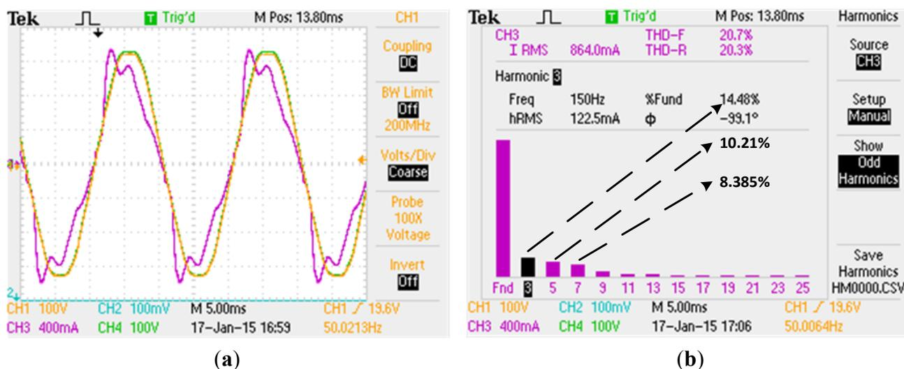
**Figure 8.** (a) Grid’s voltage and current waveforms before harmonic compensation; (b) Grid’s current harmonic spectrum before harmonic compensation.
