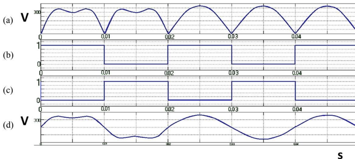
**Figure 2.** (a) Buck-boost's output voltage; (b)  $S_1$ ,  $S_4$  pulses; (c)  $S_2$ ,  $S_3$  pulses; (d) Inverter's output voltage.
