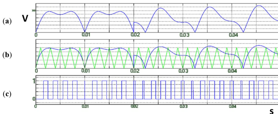
**Figure 4.** (a)  $V_{dc,out}$  created by the buck-boost converter; (b) Comparison of the resulting carrier waveform with 20 KHz reference triangle; (c) Created pulses.
