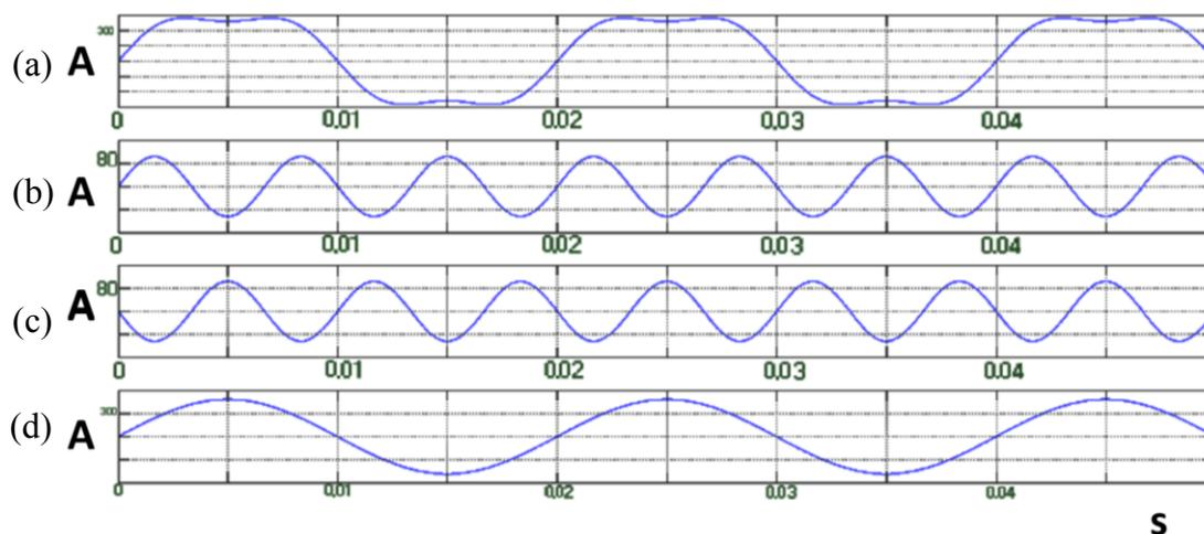
**Figure 3.** (a) Distorted ac grid's current before compensation; (b) 3rd harmonic component at the grid before compensation; (c) Mirror 3rd harmonic component injected to the PCC; (d) AC current of the grid after harmonic compensation.
