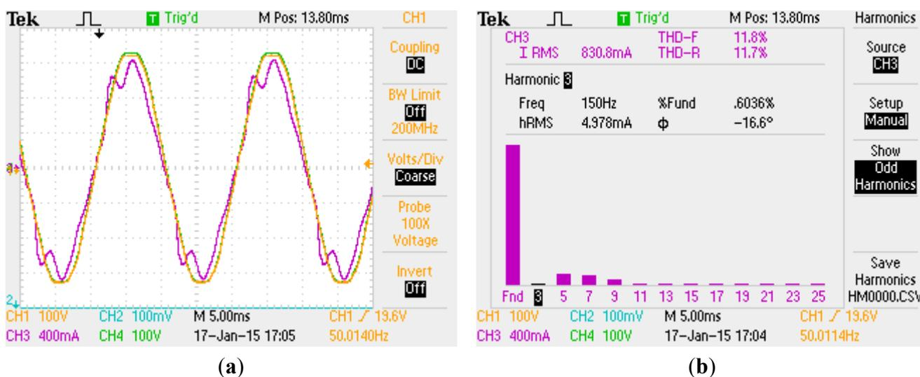
**Figure 9.** (a) Grid’s voltage and current waveforms after compensation of 3rd harmonic; (b) Grid’s current harmonic spectrum after compensation of 3rdharmonic. 3rd harmonic is shown.
