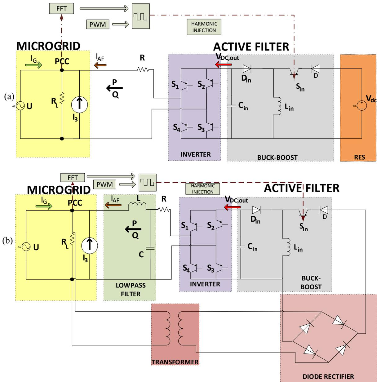
**Figure 1.** (a) Configuration of the studied system in the first case; (b) Configuration of the studied system in the second case.
