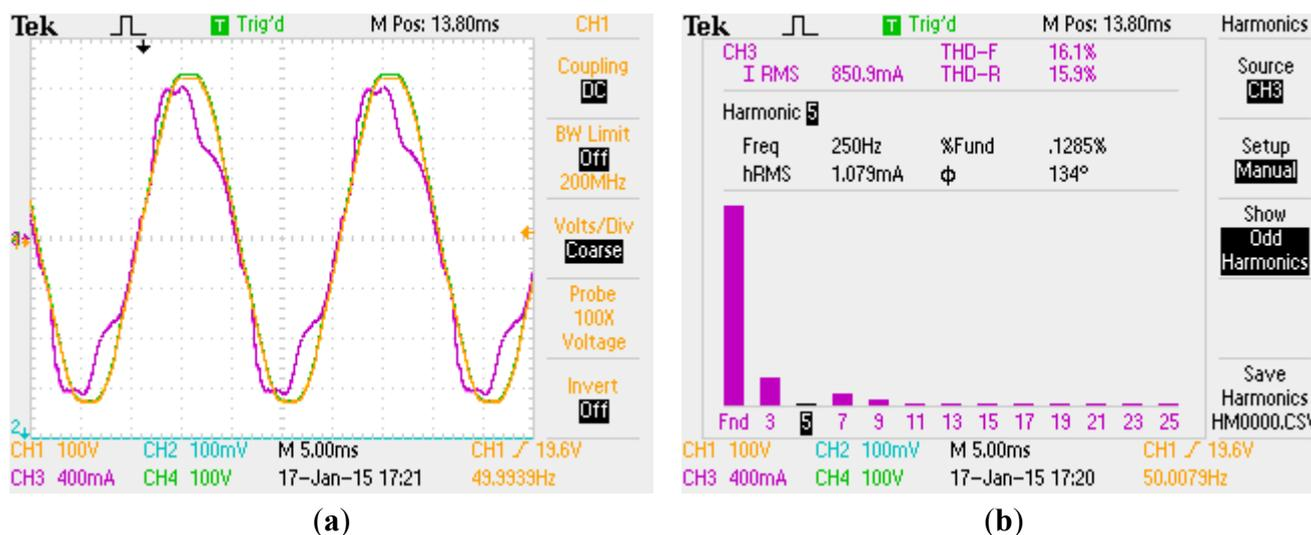
**Figure 10.** (a) Grid's voltage and current waveforms after compensation of 5th harmonic; (b) Grid's current harmonic spectrum after compensation of 5th harmonic. 5th harmonic is shown.
