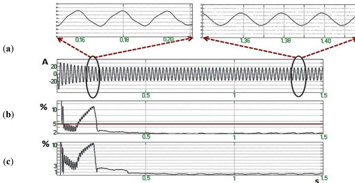
**Figure 7.** (a) Grid's current  $I_G$ ; (b) Grid's current THD; (c) Grid's current 3rd harmonic component with higher harmonics filtering.
