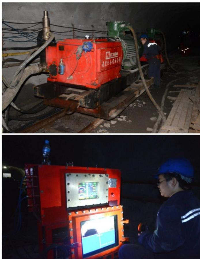
**Figure 8.** Field test of cross-measure hydraulic fracturing in underground coalmines.
