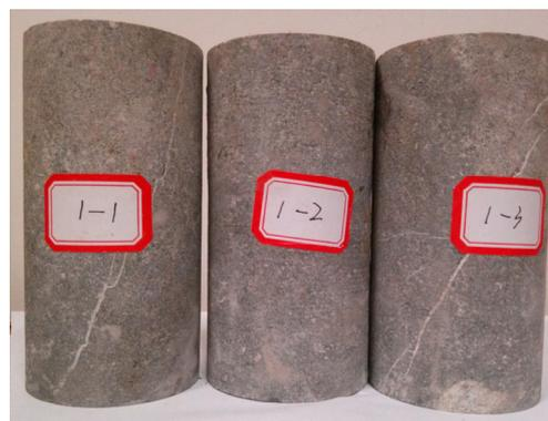
Figure 6. Specimens in acoustic emission test.
