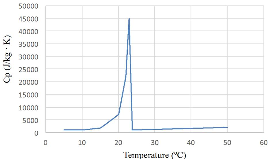
**Figure 4.** Effective heat capacity.
