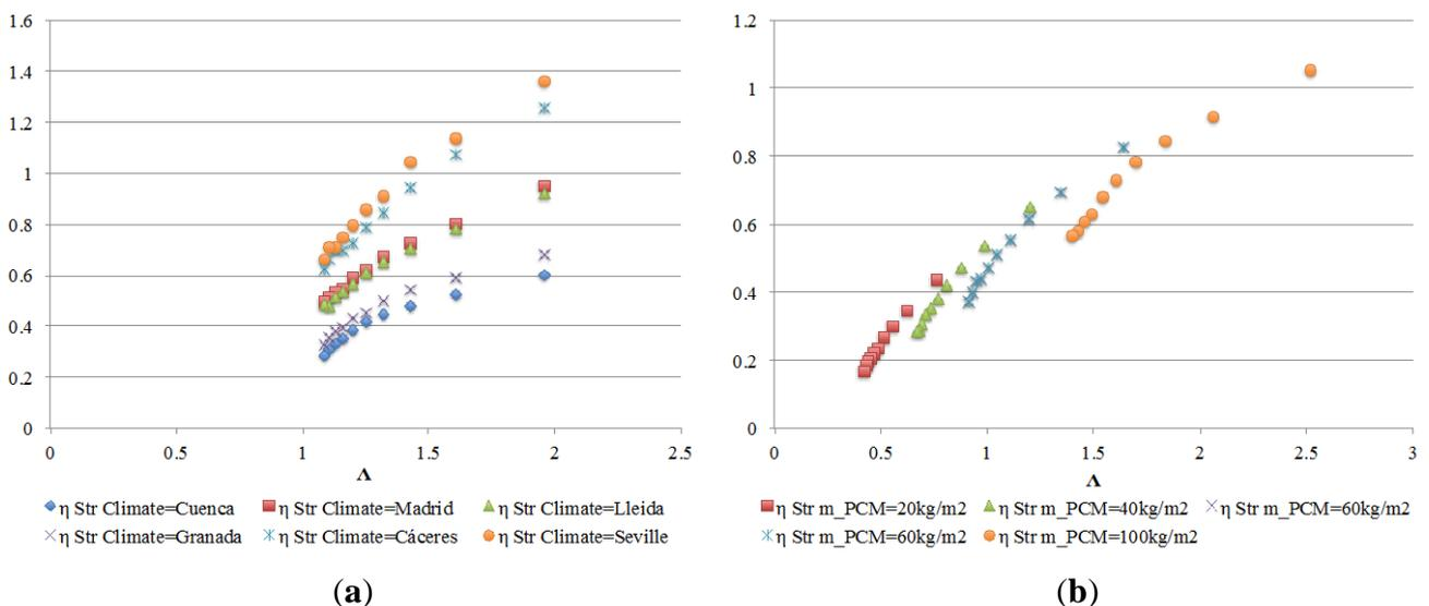
**Figure 12.** Efficiency as a regenerator: (a) different climates; (b) different amounts of PCM.
