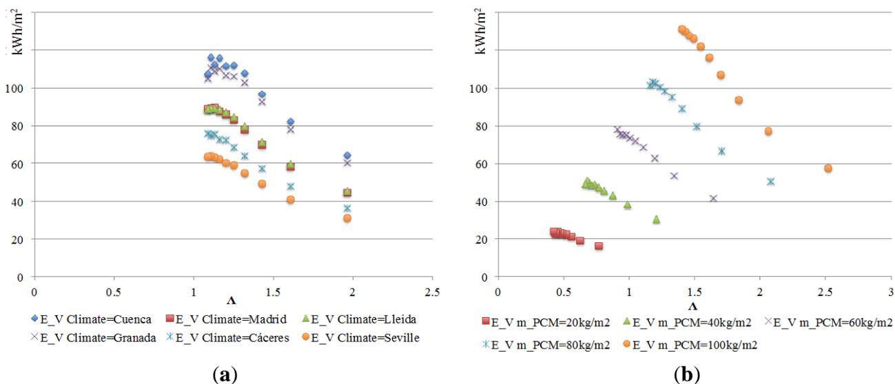
Figure 10. Ventilation energy delivered in July and August: (a) different climates; (b) different amounts of PCM.
