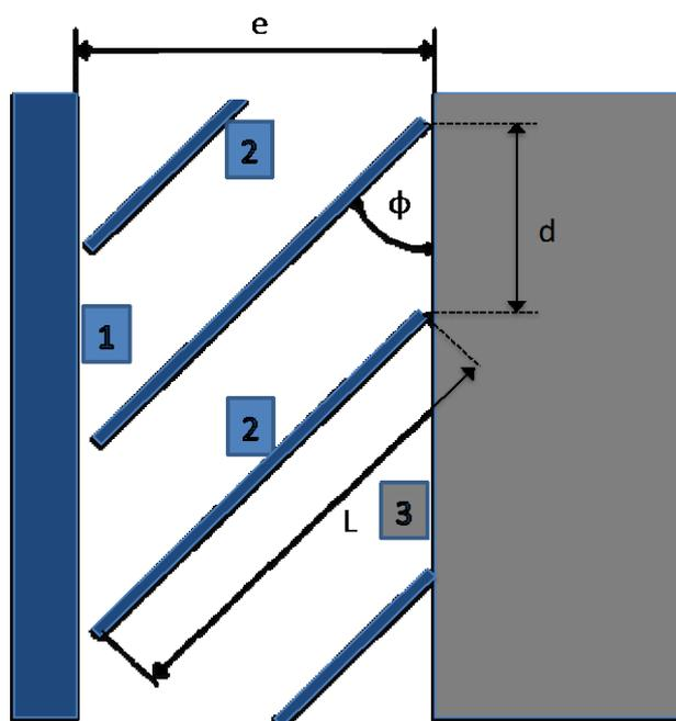
**Figure 1.** Façade diagram: plan view: (1) Outer element; (2) the fins; and (3) the inner element.
