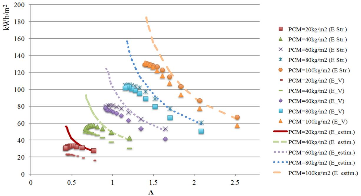
**Figure 11.** Energy stored, energy delivered for ventilation, and estimated energy storage in July and August.
