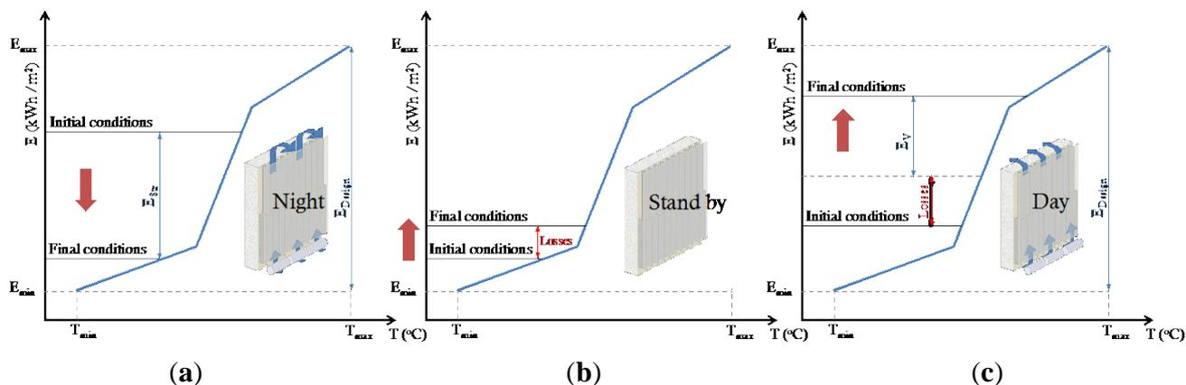
Figure 2. Façade operation: (a) Storage; (b) Standby; (c) Release.
