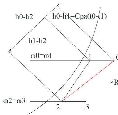
**Figure 2.** The conventional and HPHX systems compared in the psychrometric chart. Conventional system: 0-2-3; HPHX system: 0-1-2-3;  $h_{0,1,2,3}$  = air enthalpy, kJ/kg;  $w_{0,1,2,3}$  = air moisture content at the various states, kg/kg;  $C_{pa}$  = air specific heat, kJ/kg·K;  $t_0, t_1$  = air temperature, °C.
