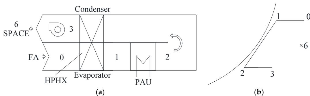
**Figure 1.** (a) The schematic diagram of the fresh air (FA) treatment with heat pipe heat exchanger (HPHX); (b) the air treatment processes of the FA with HPHX in the psychrometric chart. 0: FA; 1: pre-cooled air; 2: cooled air; 3: re-heated air; 6: space air.
