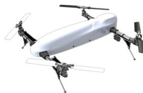
Figure 1. The variable-pitch quadrotor.
