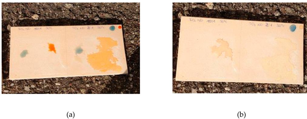
**Figure S10.** Ceramic tiles with molar ratio  $C_{12}H_{28}O_4Ti:CO(NH_2)_2$  10:1 (left part of image) and 2:1 (right part of image), 50 °C, before (a) and after (b) ½ hour of sunlight exposure.
