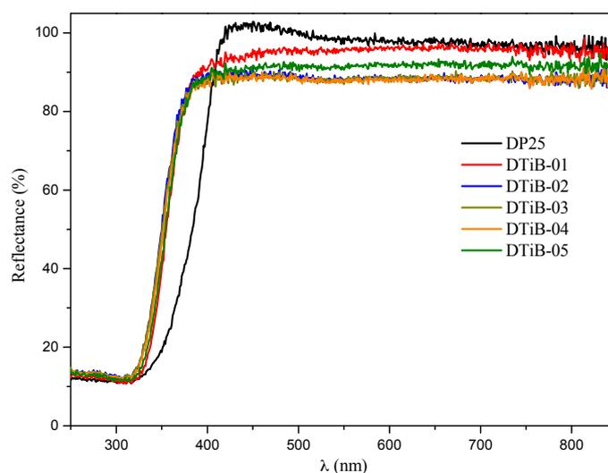
**Figure 7.** Diffuse reflectance ultraviolet-visible spectroscopy (DRS UV-vis) spectra for all the CD-aTiO<sub>2</sub> samples prepared in this work and for the commercial DP25 TiO<sub>2</sub>.
