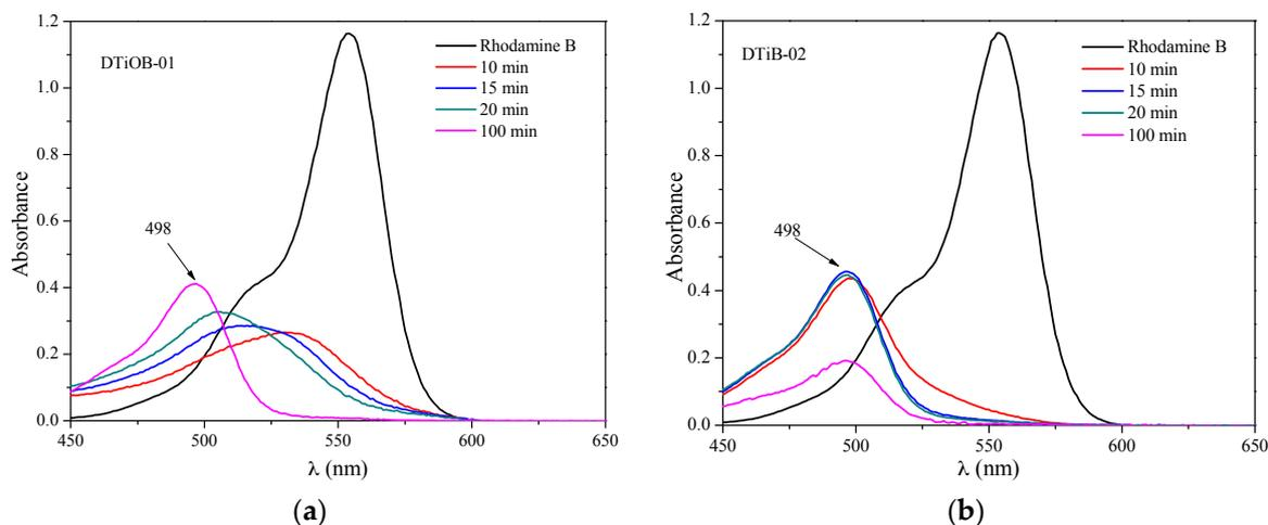
**Figure 9.** Hypsochromic shift detected during the degradation process of Rhodamine B with (a) DTiB-01 and (b) DTiB-02.
