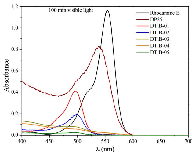
**Figure 10.** UV-Vis spectra for the remaining Rhodamine B solutions after a 100 min exposure to visible light.
