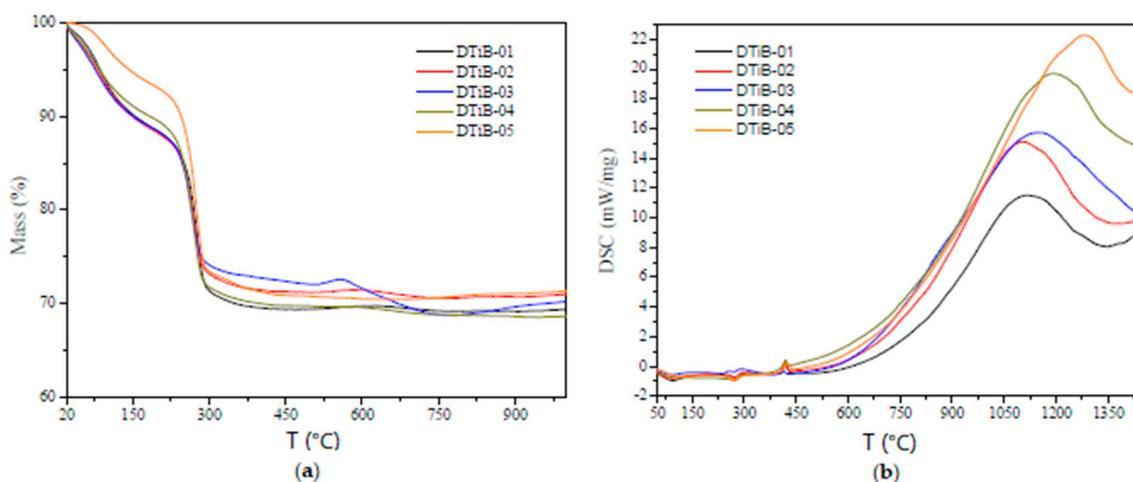
**Figure 6.** (a) Thermogravimetric (TG) and (b) differential scanning calorimetry (DSC) analysis for all the CD-aTiO<sub>2</sub> photocatalysts synthesized and used in this work.
