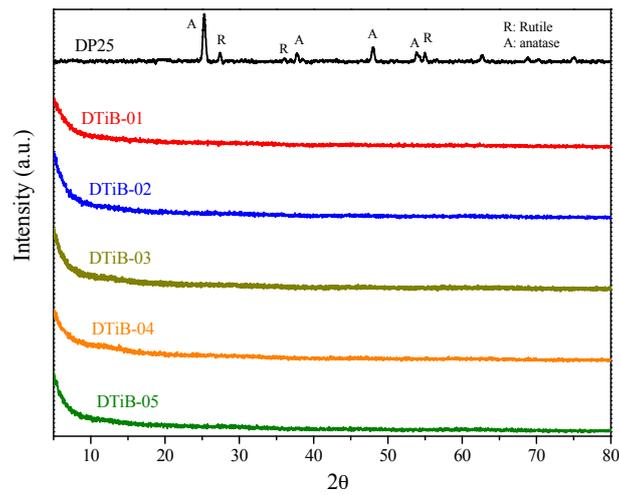
**Figure 1.** X-ray diffractograms of all the obtained aTiO<sub>2</sub> and commercial DP25 products.
