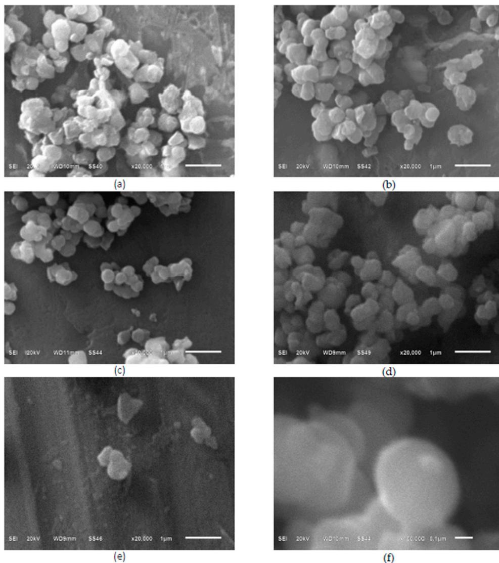
**Figure 2.** Scanning electron microscope (SEM) micrographs of all the CD-aTiO<sub>2</sub> prepared (a) DTiB-01; (b) DTiB-02; (c) DTiB-03; (d) DTiB-04; (e) DTiB-05; (f) the disc morphology with a dimension of ~300 nm in diameter of these products can be observed in the last pictured.
