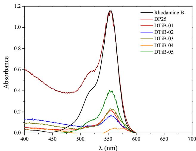
**Figure 8.** UV-Vis spectra of the final concentration of Rhodamine B after a 20 min adsorption process in the presence of all the photocatalysts.
