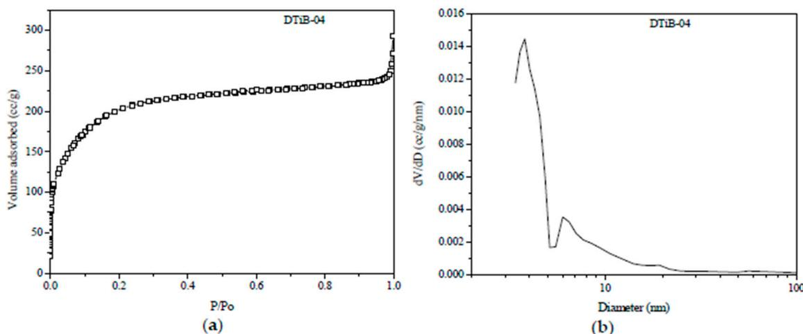
**Figure 4.** (a) N<sub>2</sub> adsorption-desorption plot for the DTiB-04 isotherm; (b) Pore size distribution curve for the same DTiB-04 sample obtained from the desorption isotherm.
