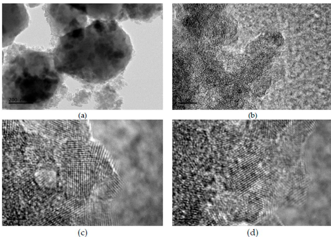
**Figure 3.** Transmission electron microscope (TEM) images of carbon-coated CD-a $\text{TiO}_2$  for the DTiB-04 photocatalyst, (a) particles conglomerates at 200 nm (see Figure 1b), (b) zoom of image (a) to 5 nm and (c,d) nanocrystals of image (b) to 2 nm.
