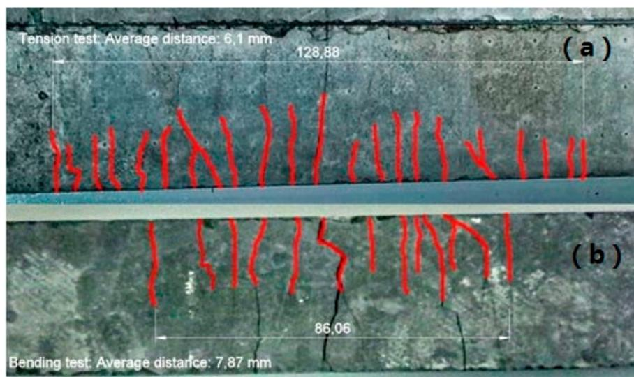
**Figure 6.** Cracking maps of two composites from the same plate tested under tensile (a) and bending test (b).
