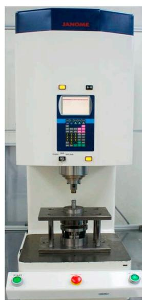
Figure 8. The electro press for the micro-channel array forming process (JANOME JP-5004).
