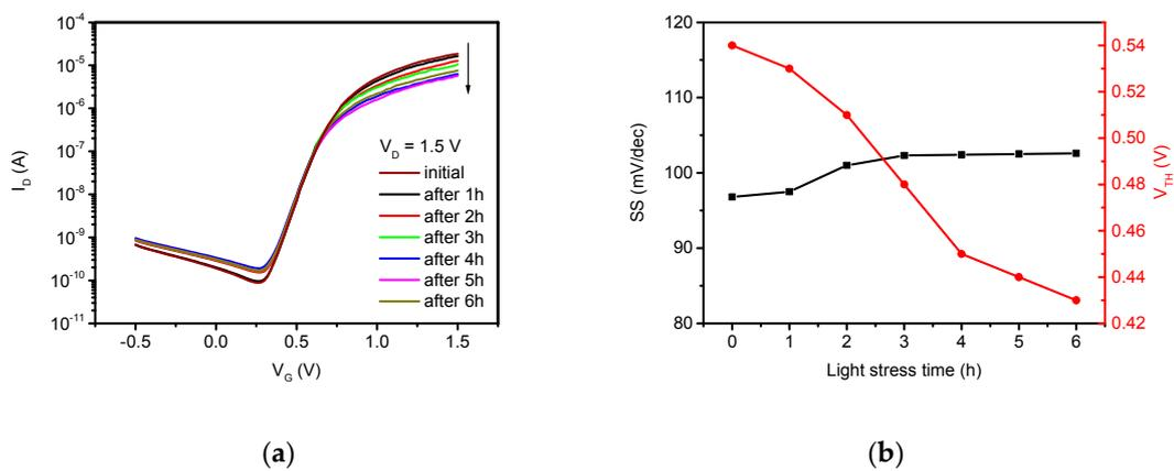
Figure S2. (a) Transfer characteristics, (b) threshold voltage and subthreshold swing of the TFT after white-light stress (around 2000 lx) for several durations.
