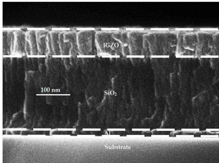
Figure S1. Cross-sectional SEM image of the sputtered SiO<sub>2</sub> electrolyte.
