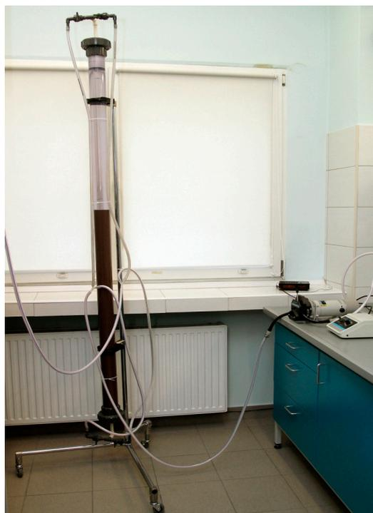
Figure 1. Ion-exchange column for the production of  $\text{Ni}(\text{ReO}_4)_2$ .
