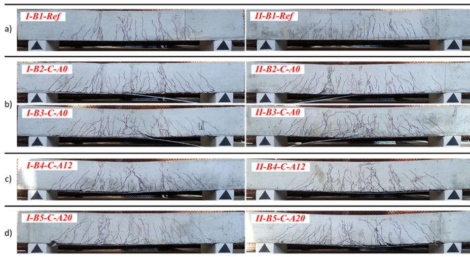
Figure 14. Crack pattern of the beams: (a) reference; (b) with pure adhesive bond; (c) with  $2 \times 6$  pins; (d) with  $2 \times 10$  pins.
