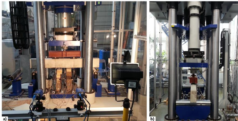
Figure 9. Beam tests: (a) test setup with high-speed cameras; (b) loading frame.
