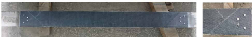
Figure 4. Hybrid jointing using  $2 \times 4$  pins.
