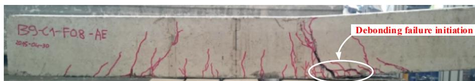
Figure 5. Failure of a beam with hybrid jointing using  $2 \times 4$  pins [23].
