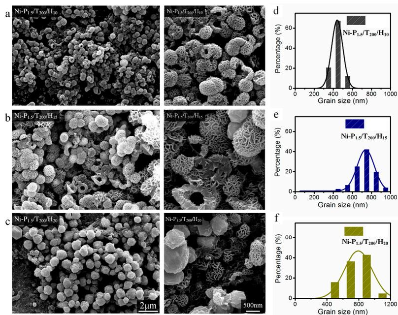
**Figure 2.** SEM images and corresponding particle size distributions of Ni-P<sub>1.5</sub>/T<sub>200</sub>/H<sub>10</sub> (a,d), Ni-P<sub>1.5</sub>/T<sub>200</sub>/H<sub>15</sub> (b,e), and Ni-P<sub>1.5</sub>/T<sub>200</sub>/H<sub>20</sub> (c,f) powders. The scale bars apply to all images in a column.
