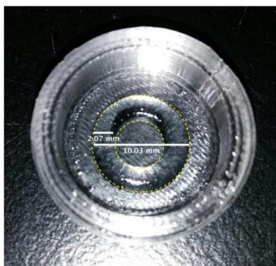
**Figure 5.** Representative printed ring in MC-Na005 hydrogel in the M12 support. The inner and outer diameters are shown by dotted lines.
