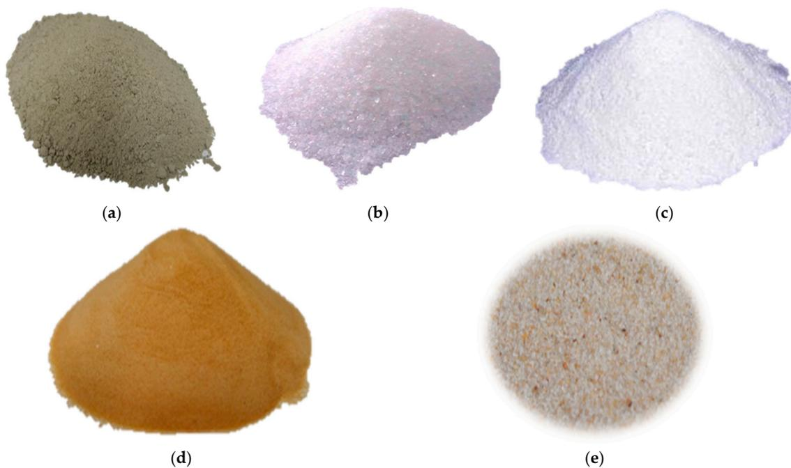
**Figure 1.** The raw materials: (a) cement blend; (b) citric acid; (c) zinc acetate; (d) redispersible polymer powder; and (e) quartz sand.
