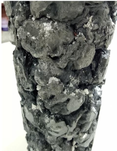
**Figure 7.** Crystals produced on surface of cementless specimen.
