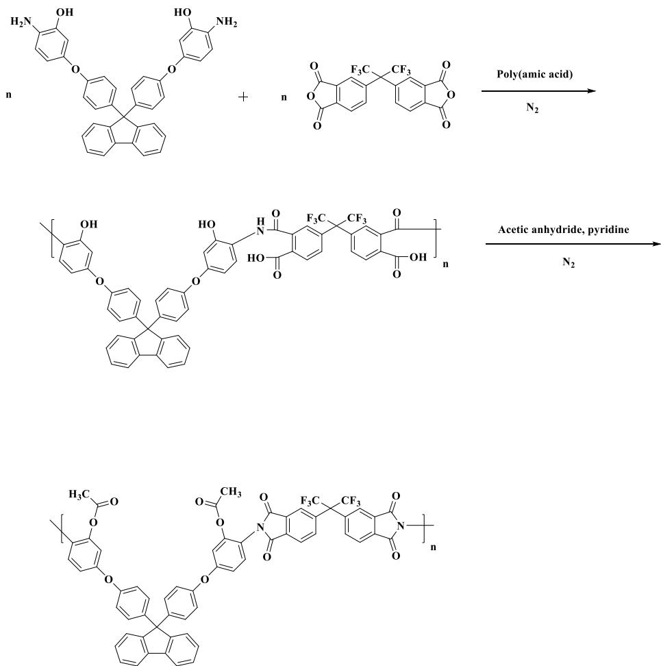
**Figure S4.** Synthesis procedures of polyimide.
