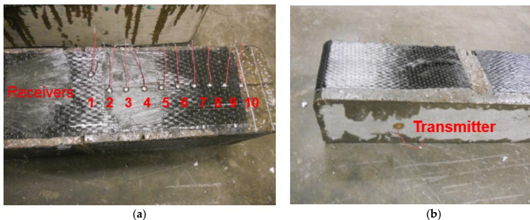
**Figure 4.** Sensors on beam 2: (a) front view (b) back view.
