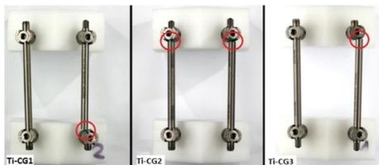
**Figure 3.** Sites of rod fracture of titanium control group (Ti-CG) post biomechanical testing and fatigue fractures of the rods at the rod-screw junction.
