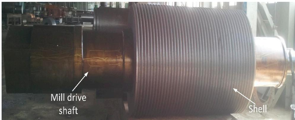
**Figure 1.** Sugar mill roller shaft with final groove ready for shipment.
