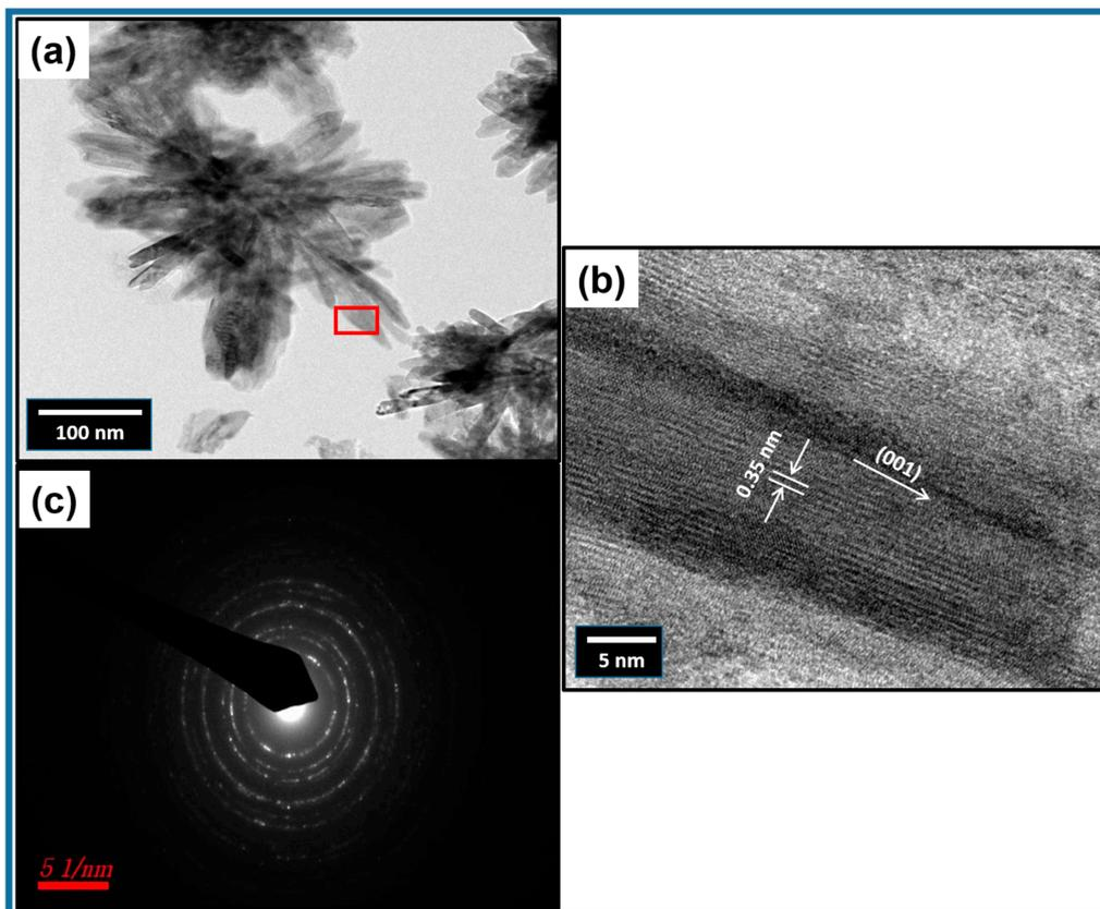
**Figure 3.** Typical (a) TEM, (b) HRTEM, and (c) SAED pattern of TiO<sub>2</sub> nanoflowers synthesized by facile low-temperature solution process.
