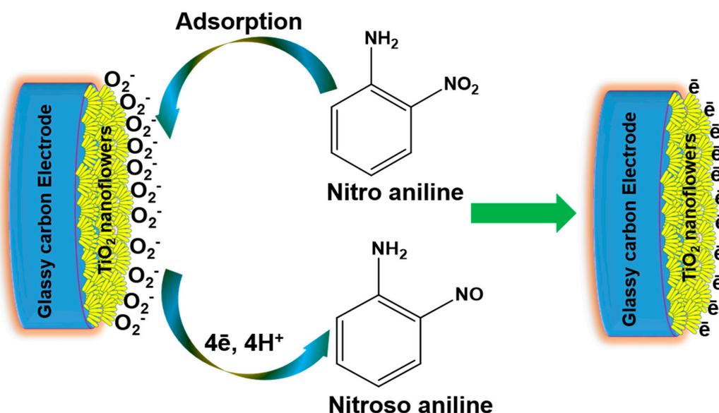
**Figure 9.** Illustration of possible nitroaniline chemical sensing over TiO<sub>2</sub> nanoflowers-modified glassy carbon electrode (GCE).
