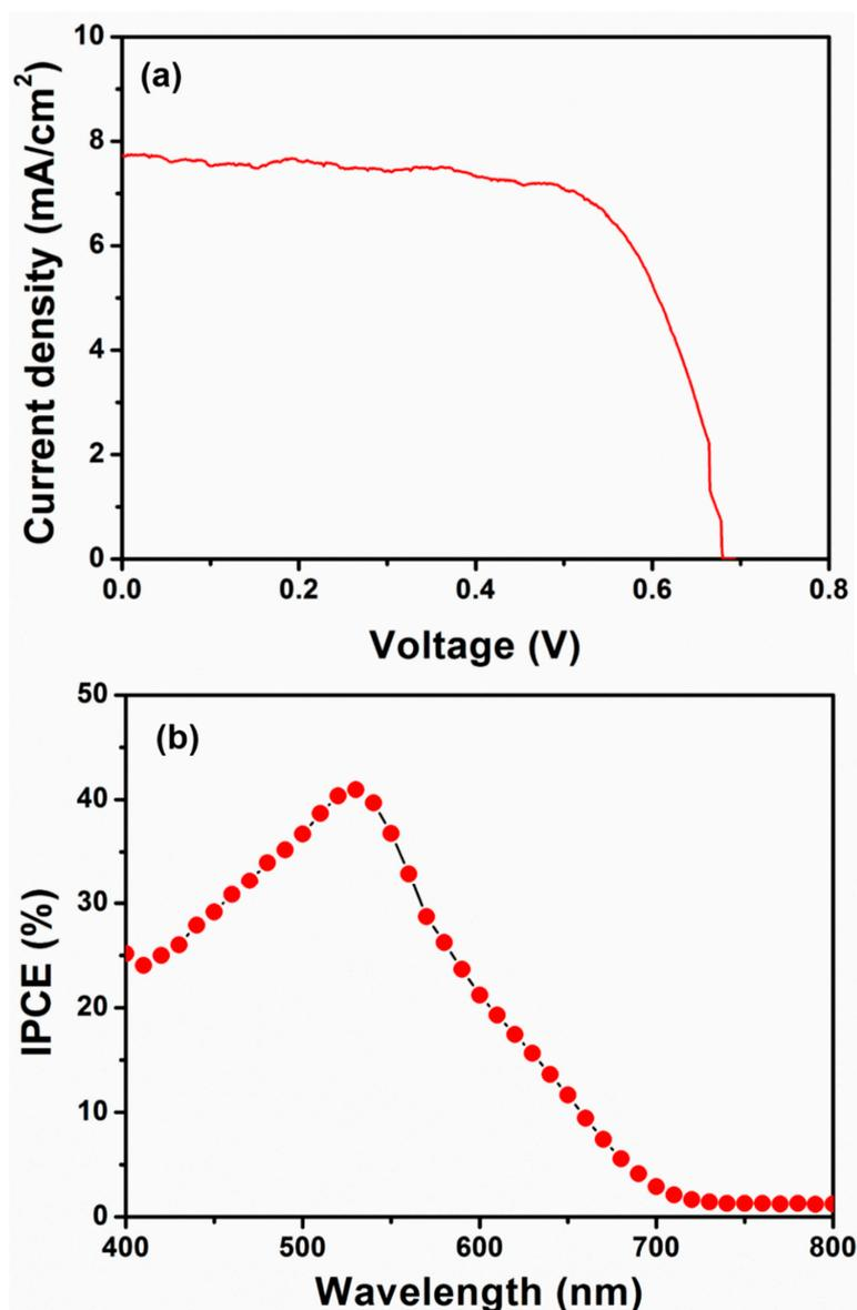
**Figure 7.** Typical (a) current–voltage (J–V) and (b) incident photon to current efficiency (IPCE) characteristics of TiO<sub>2</sub> nanoflowers-based dye-sensitized solar cells.
