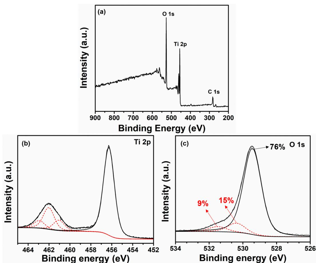
**Figure 5.** Typical XPS spectra of (a) survey, (b) deconvoluted high-resolution Ti 2p, and (c) deconvoluted high-resolution O 1s plots of as-synthesized TiO<sub>2</sub> nanoflowers.
