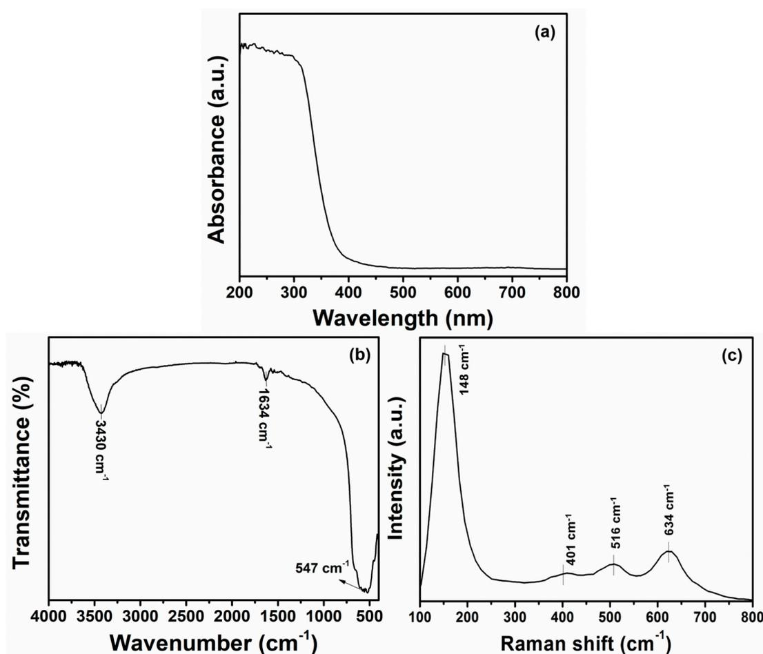
**Figure 4.** Typical (a) UV–Visible, (b) FTIR, and (c) Raman-scattering spectroscopy of synthesized TiO<sub>2</sub> nanoflowers.
