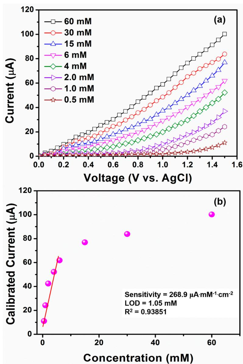
**Figure 8.** Typical (a) concentration-dependent (concentrations of 60–0.5 mM in 0.1 M PBS) I–V response of the fabricated  $\text{TiO}_2$  nanoflowers-based nitroaniline chemical sensor; (b) corresponding graph for calibration current vs. concentration of nitroaniline.
