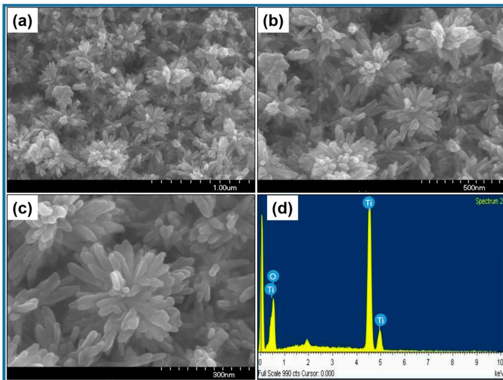
**Figure 2.** (a–c) FESEM images and (d) EDS spectrum of TiO<sub>2</sub> nanoflowers synthesized by facile low-temperature solution process.
