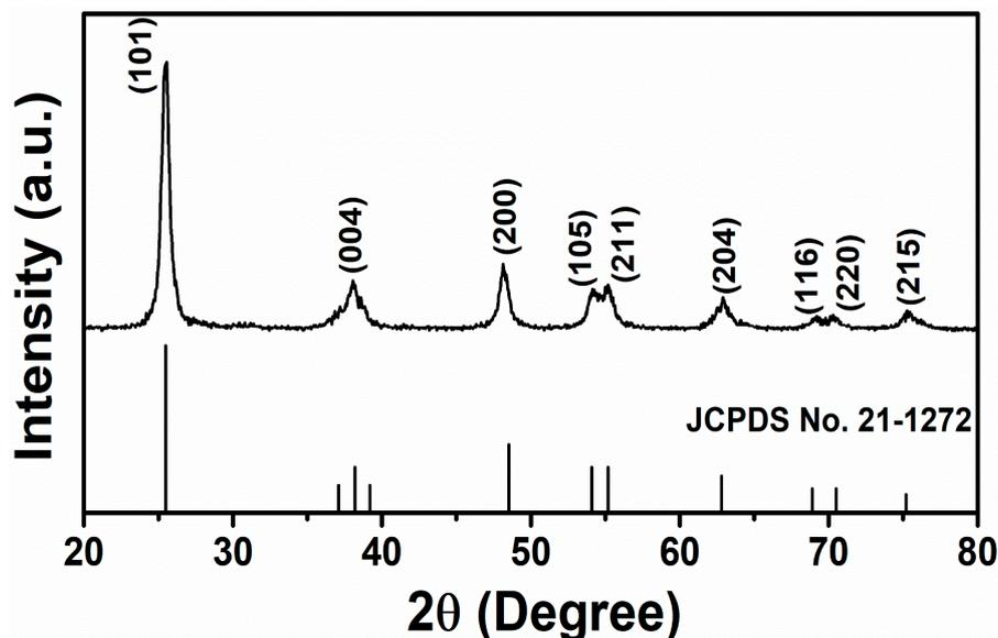
**Figure 1.** Typical XRD patterns of TiO<sub>2</sub> nanoflowers synthesized by facile low-temperature solution process.
