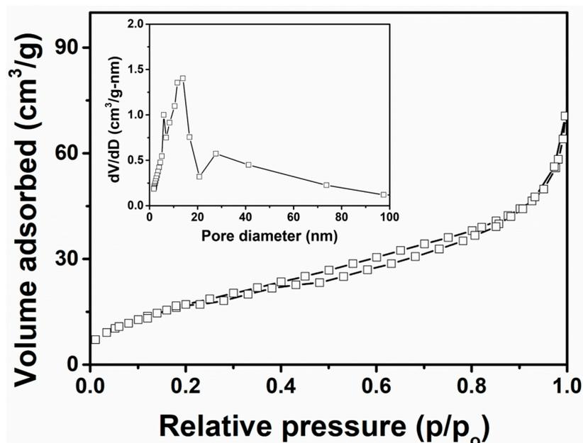
**Figure 6.** Nitrogen adsorption–desorption isotherms and pore-size distributions (inset) of as-synthesized TiO<sub>2</sub> nanoflowers.
