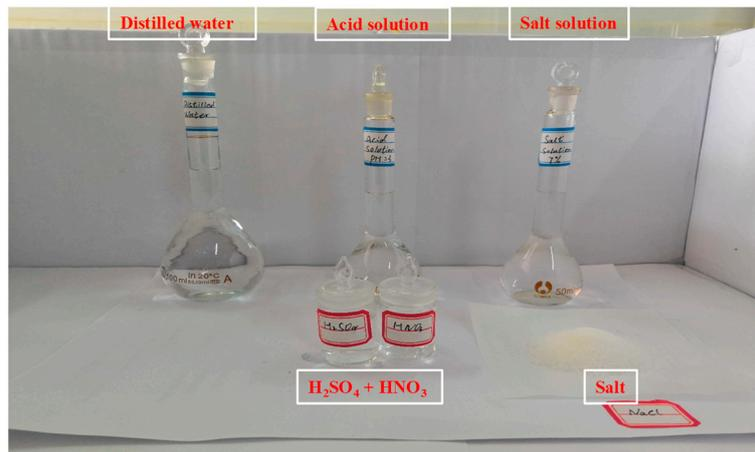
Figure 1. Simulated environment reagents.
