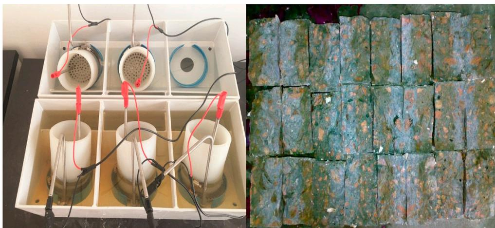
**Figure 6.**  $\text{Cl}^-$  penetration device and testing specimens.
