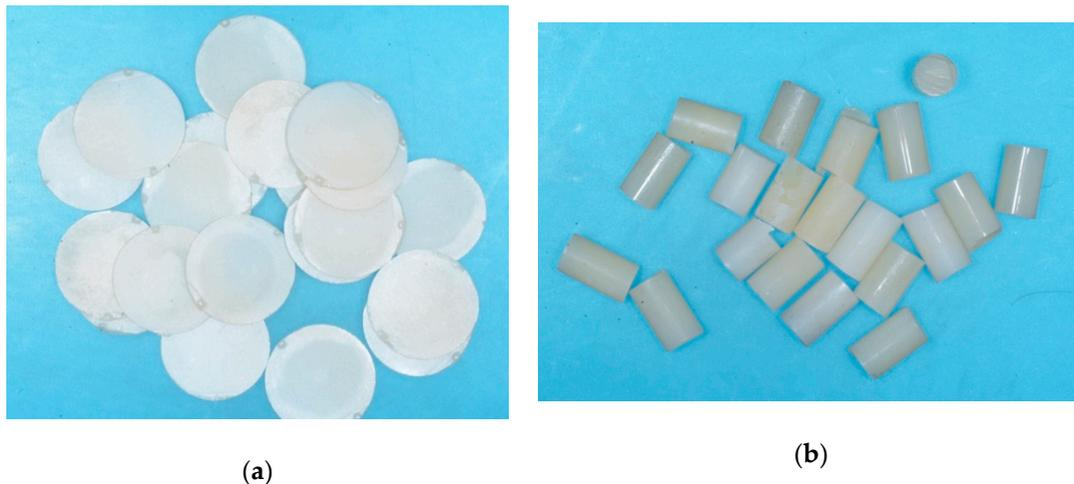
**Figure 1.** (a) Y-TZP disks used for the study (10 mm diameter, 0.5 mm thick) (n = 20); (b) Nano-hybrid composite cylinders created for the study (4 mm diameter, 8 mm height) (n = 20).
