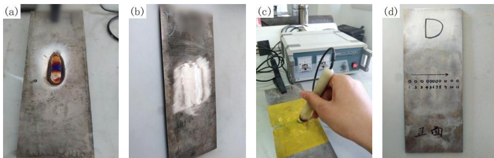
Figure 4. Specimens pre-treatment before X-ray diffraction (XRD): (a) before polished; (b) after polished; (c) electrochemical polishing; and (d) labeling measure point.
