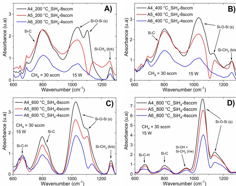
**Figure 3.** IR spectra for the a-Si<sub>1-x</sub>C<sub>x</sub>:H films deposited after fast annealing process with different R<sub>0</sub> ratios (from 37.5–75) and constant RF power at 15 W; upon fast annealing process at 200 (A), 400 (B), 600 (C), and 800 °C (D).
