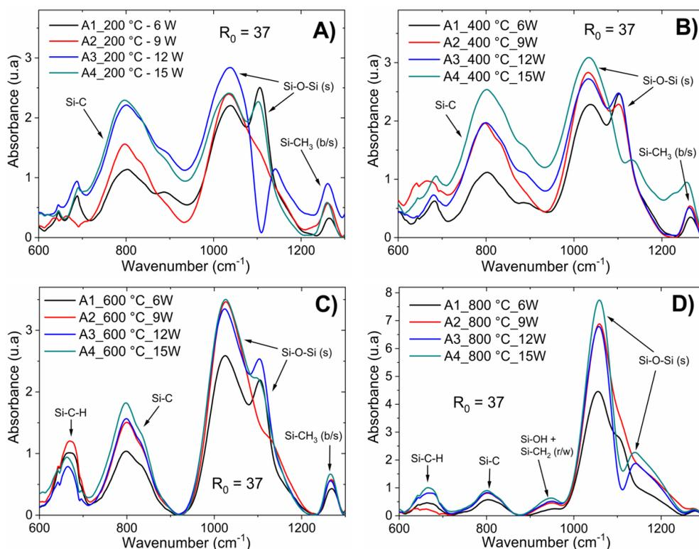
**Figure 2.** IR spectra for the a-Si<sub>1-x</sub>C<sub>x</sub>:H films deposited after fast annealing process with different RF power (from 6–15 W) while keeping the CH<sub>4</sub>/SiH<sub>4</sub> ratio constant; upon fast annealing process at 200 (A), 400 (B), 600 (C), and 800 °C (D).
