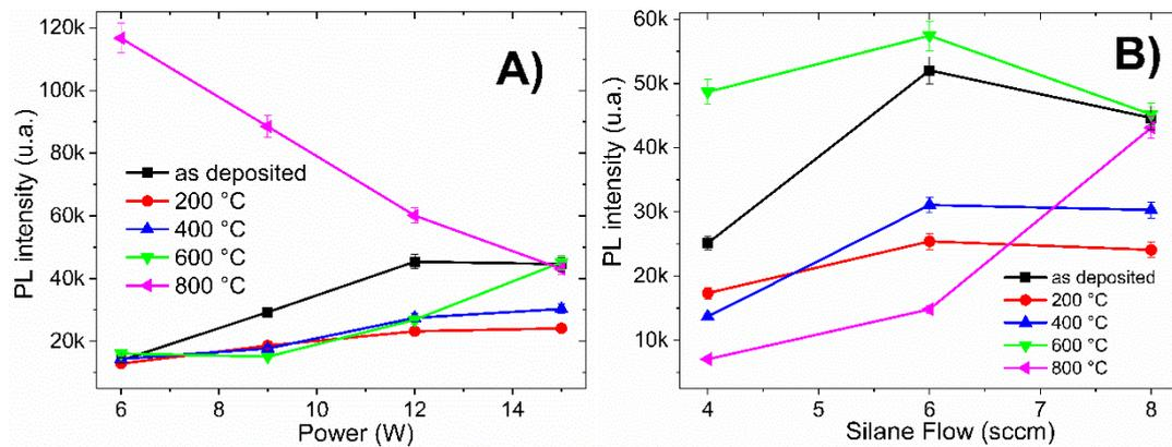
**Figure 8.** PL intensity of a-Si<sub>1-x</sub>C<sub>x</sub>:H films deposited: (A) with different RF power (6–15 W) maintaining constant  $R_0$  ratio (37.5); and (B) with different  $R_0$  ratios (37.5–75) and fixed RF power (15 W).
