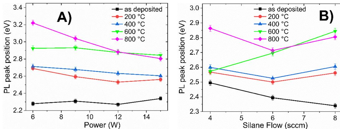
**Figure 7.** PL peak position of a-Si<sub>1-x</sub>C<sub>x</sub>:H films deposited: (A) with different RF power (6–15 W) keeping the ratio  $R_0$  constant (37.5); and (B) with different  $R_0$  (37.5–75) with constant RF power (15 W).
