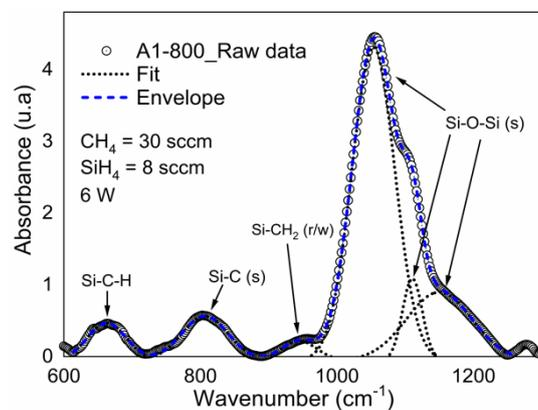
**Figure 4.** Deconvolution of A1 sample (6 W and R<sub>0</sub> = 37.5) upon fast annealing process at 800 °C.
