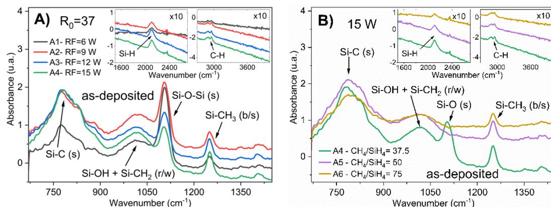
**Figure 1.** FTIR spectra of as-deposited a-Si<sub>1-x</sub>C<sub>x</sub>:H films: (A) with different RF power (6–15 W) at a constant ratio of CH<sub>4</sub>/SiH<sub>4</sub> (R<sub>0</sub> = 37.5); and (B) corresponding to films deposited with different CH<sub>4</sub>/SiH<sub>4</sub> ratios (R<sub>0</sub> from 37.5 to 75) with a constant RF power of 15 W.
