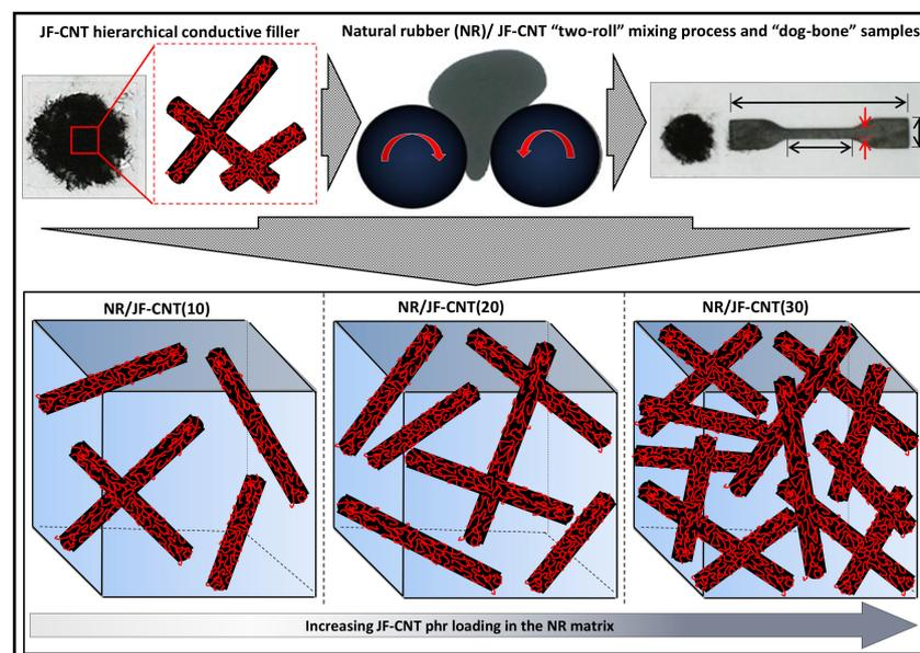
**Figure 1.** Schematic illustration of the two-roll mixing process for the fabrication of NR/JF-CNT composites and the resulting composites at different phr loadings. The final dog-bone shaped samples used for the tensile test experiments (dimensions of the samples according to the ASTM D412 (D 412) Tensile Strength Properties of Rubber and Elastomers, as well as the electrical conductivity and thermoelectric measurements are also depicted.
