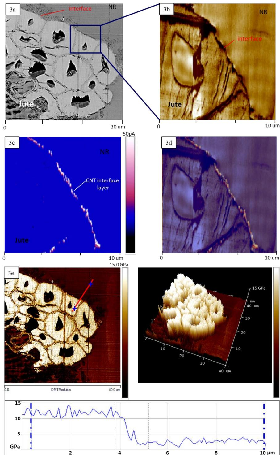
**Figure 3.** (a,b) Atomic force microscopy (AFM) phase images, (c) PeakForce TUNA current map of single JF-CNT/NR cross-section (scale: 50 pA,  $V_{bias} = 5$  V) and (d) the overlay of Figure 3b,c images; (e) 2D and 3D peak force tapping quantitative nanomechanical (PFT-QNM) analysis of Derjaguin–Muller–Toporov (DMT) modulus map over the NR/JF-CNT cross-section and the corresponding section analysis (indicated red line).
