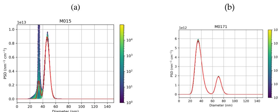
**Figure S2.** Best fitting model function obtained from SAXS analysis (red lines) with the heat map of possible PSDs calculated by taking the uncertainty and covariance of fitted parameters into account for the (a) M015 and (b) M0171 samples.
