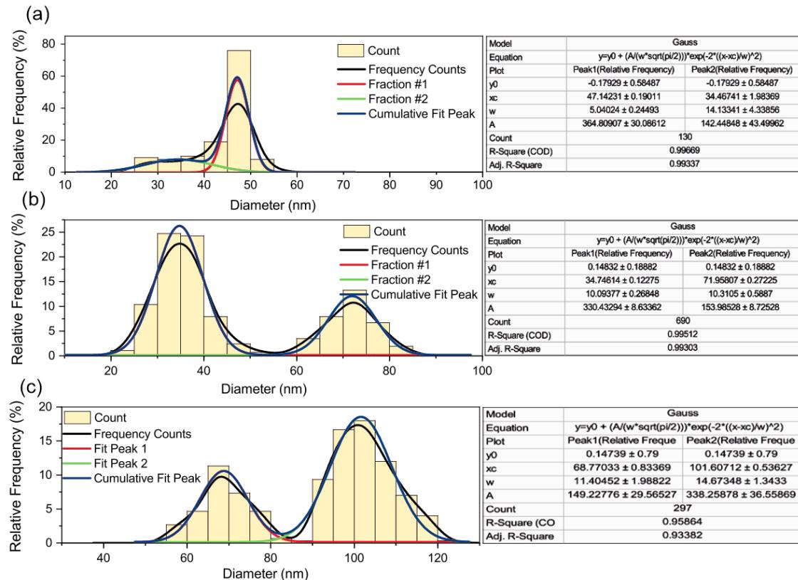
**Figure S1.** PSD as determined by TEM for the (a) M015, (b) M0171 and (c) SNP022 samples together with fitted Gaussian functions. The parameters of the best fitting model functions are summarized next to the PSDs.
