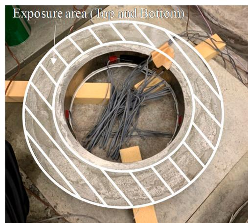
Figure 6. Restrained shrinkage (ring test).
