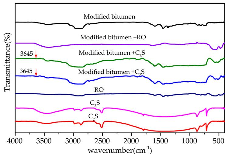
**Figure 14.** FT-IR of mixtures of bitumen–mineral components of steel slag.
