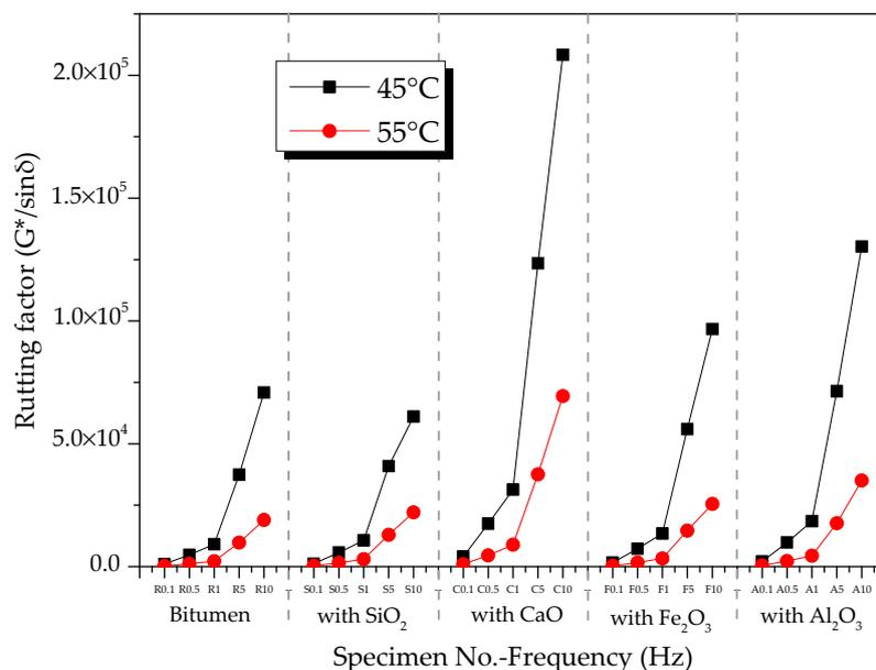
**Figure 7.** Effects of temperature on rutting factors of oxide-modified bitumen mixtures.
