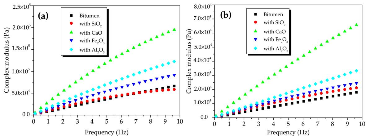
**Figure 4.** Complex shear modulus of oxide component-modified bitumen mixtures at different temperatures: (a) 45 °C and (b) 55 °C.
