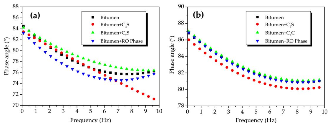
**Figure 9.** Phase angles of mixtures of modified bitumen and mineral components of steel slag ( $\text{C}_2\text{S}$ ,  $\text{C}_3\text{S}$ , and RO) at different temperatures: (a)  $45\text{ }^\circ\text{C}$  and (b)  $55\text{ }^\circ\text{C}$ .
