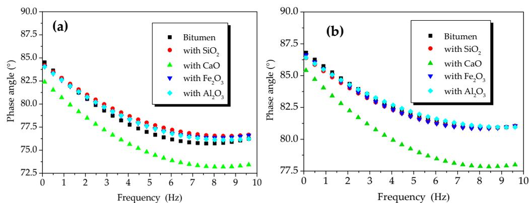
**Figure 3.** Phase angles of oxide component-modified bitumen mixtures at different temperatures: Phase angle at (a) 45 °C and (b) 55 °C.
