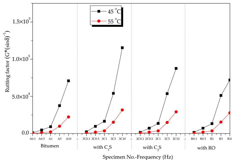
Figure 13. Effect of temperature on rutting factors of mineral phase-bitumen mixtures.
