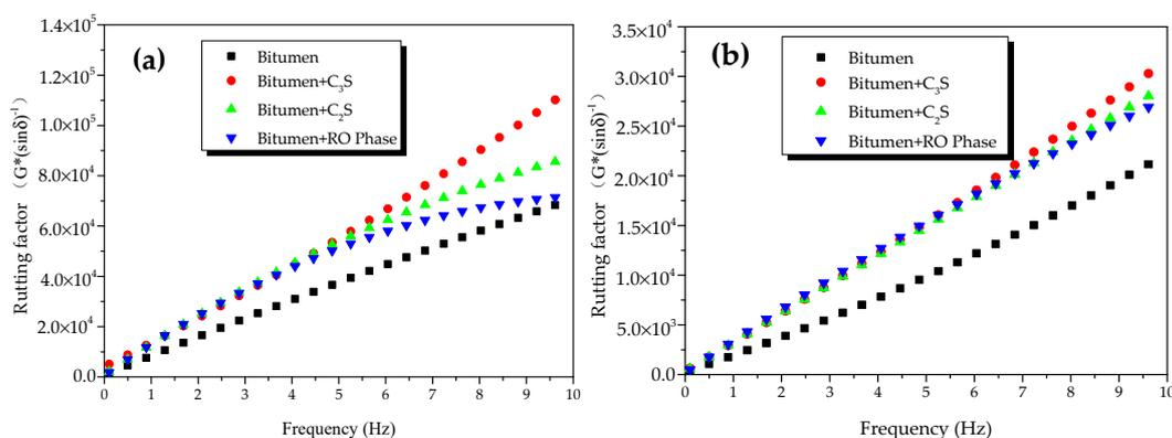
**Figure 12.** Rutting factors of bitumen–mineral mixtures at different temperatures: (a) 45 °C and (b) 55 °C.
