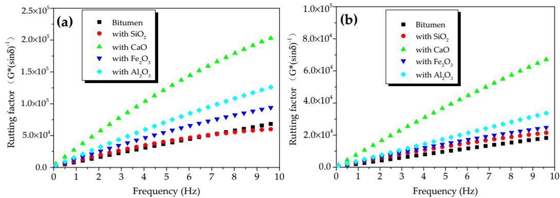
**Figure 6.** Rutting factors of oxide-modified bitumen mixtures at different temperatures: (a) 45 °C and (b) 55 °C.
