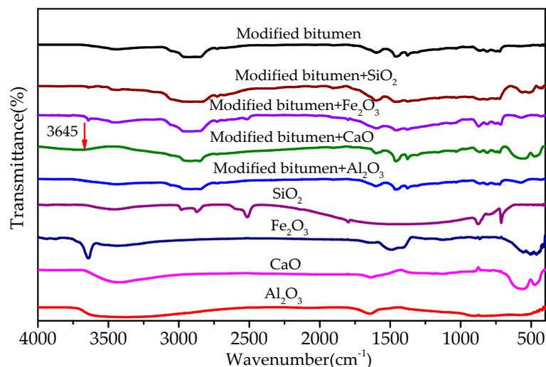
**Figure 8.** FT-IR results of mixtures of modified bitumen and chemical components of steel slag.
