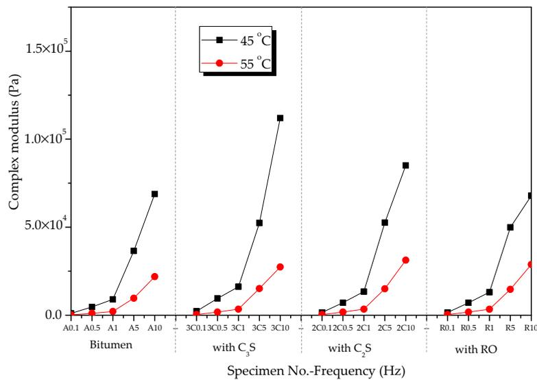
**Figure 11.** Complex shear modulus of mixtures of bitumen–mineral components of steel slag at different temperatures.
