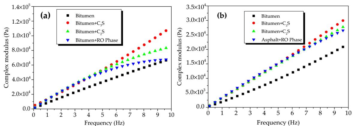
**Figure 10.** Complex shear modulus of mixtures of bitumen–mineral components of steel slag at different temperatures: (a) 45 °C and (b) 55 °C.
