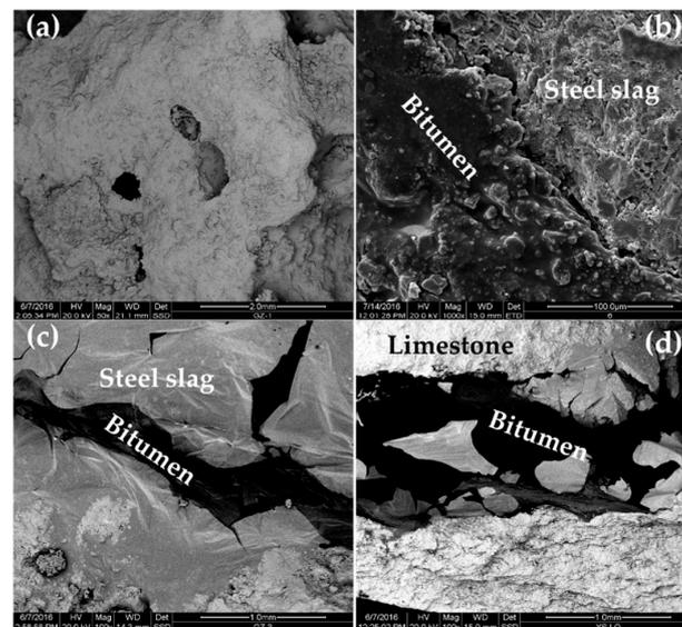
**Figure 15.** SEM images: (a) steel-slag aggregate; (b) permeable steel-slag–bitumen mixture; (c) steel-slag–bitumen sandwich interface; and (d) limestone–bitumen sandwich interface.
