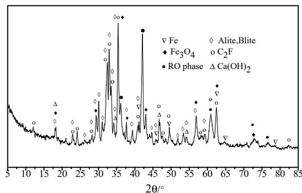
**Figure 1.** XRD test results of steel-slag aggregate.
