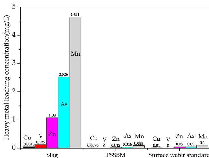
**Figure 2.** Toxic leaching of steel slag and PSSBM.
