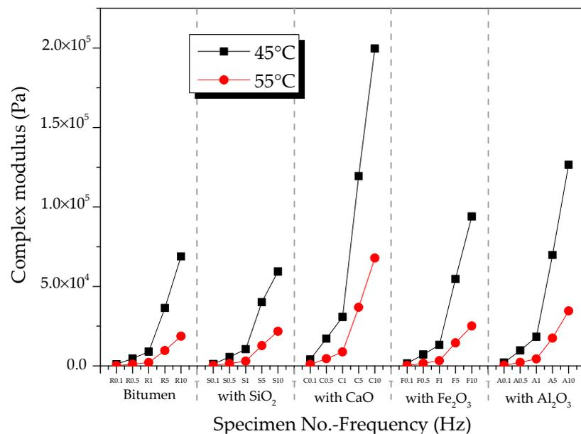
**Figure 5.** Effects of temperature on complex shear modulus of modified bitumen–oxide mixtures.
