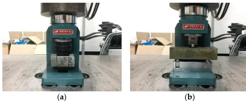
**Figure 2.** Pictures of the strength tests, with (a) the compressive strength test and (b) the flexural strength test.
