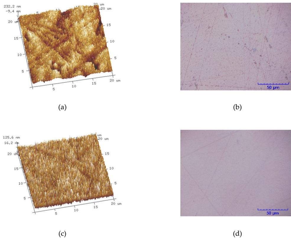
**Figure 13.** Ra and surface macro-morphology of X-cut and Z-cut. (a) Ra of X-cut (Ra 64 nm); (b) surface morphology of X-cut; (c) Ra of Z-cut (Ra 35 nm); (d) surface morphology of Z-cut.
