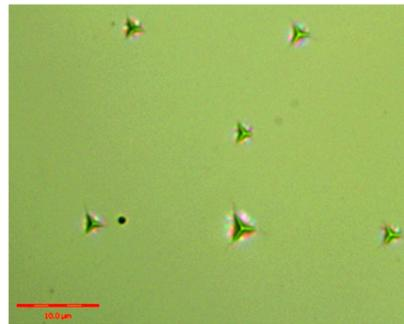
Figure 6. The indentation morphology by nano-indentation experiments.
