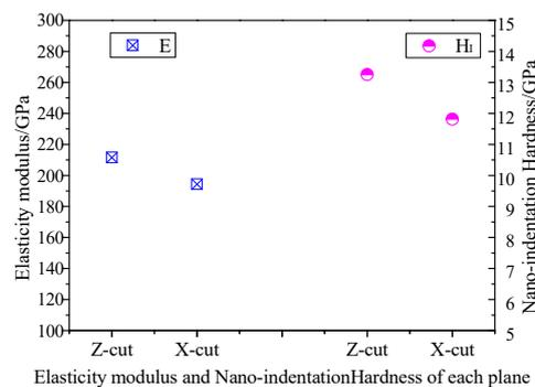
Figure 7. Elastic modulus and nano-indentation Hardness of LN.
