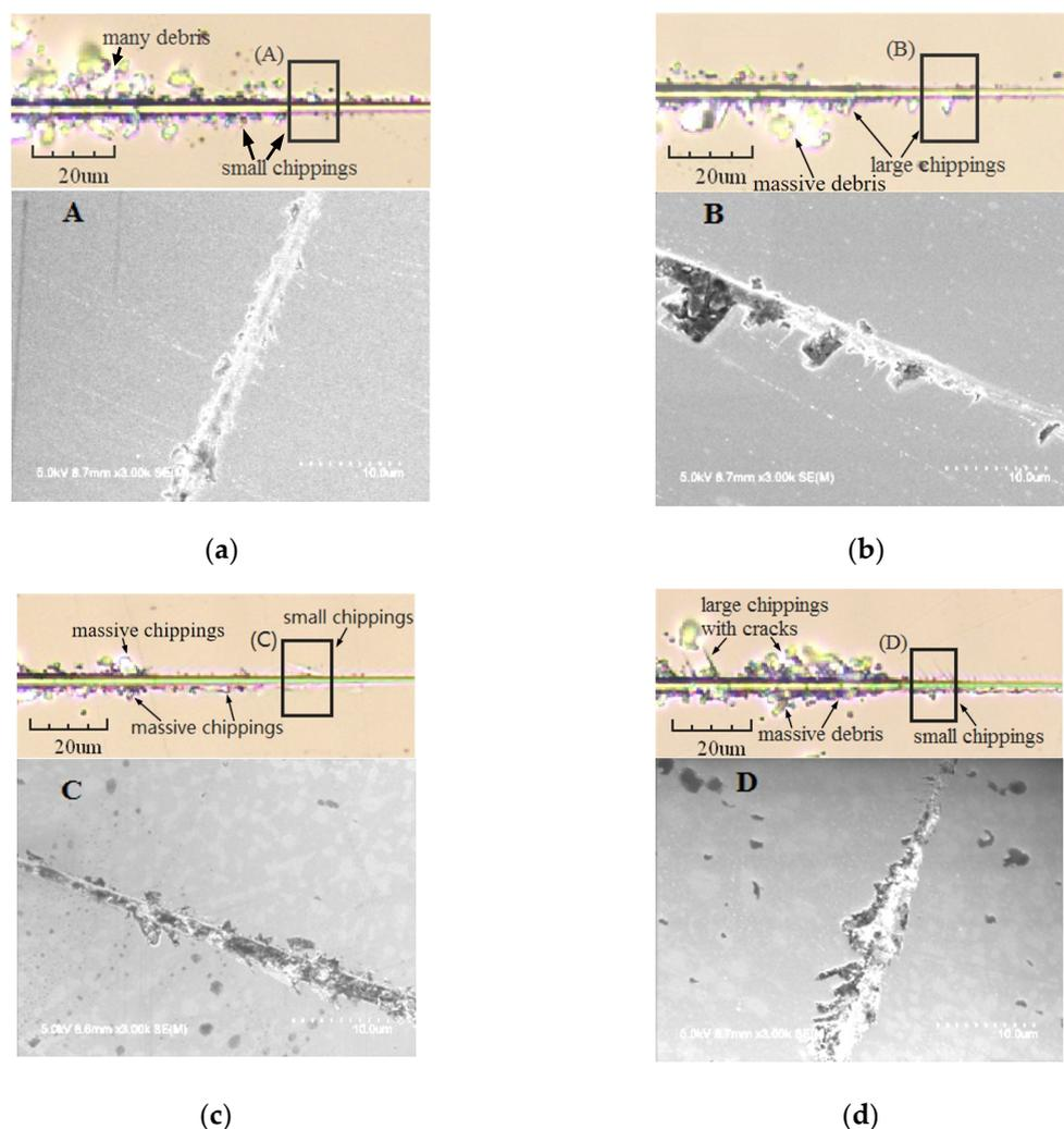
**Figure 10.** Scratches in suit scanning and SEM part magnification: (a) X axis on Z-cut, (b) Y axis on Z-cut, (c) Y axis on X-cut, (d) Z axis on X-cut.
