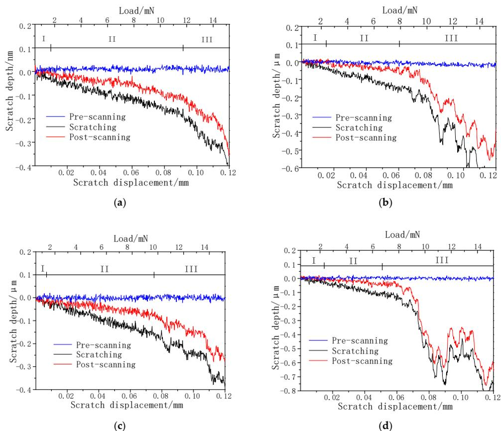
**Figure 9.** Scratch depth-displacement-load along different orientations: (a) X axis on Z-cut, (b) Y axis on Z-cut, (c) Y axis on X-cut, (d) Z axis on X-cut, of pre-scanning (I represents the elastic deformation stage, II represents the ductile deformation stage, and III represents the brittle deformation stage.).
