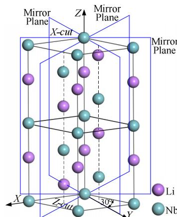
**Figure 11.** Slip orientations (X axis) in LN cell unit.
