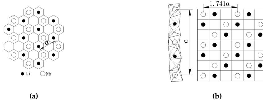
**Figure 8.** Schematic illustration of atomic structure of LN:(a) Z-cut, (b) X-cut
