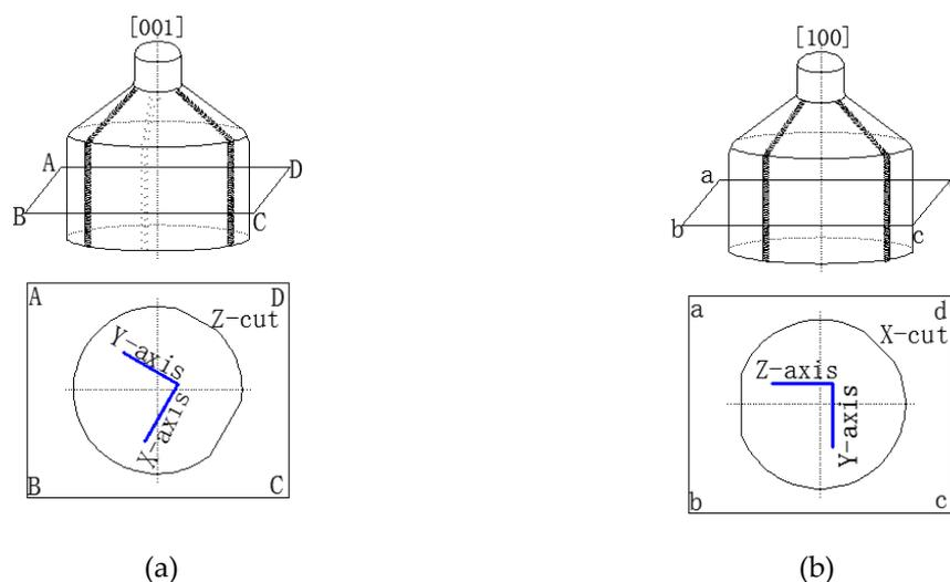
Figure 2. Scratching directions on LN different crystal wafers: (a) Z-cut, (b) X-cut.
