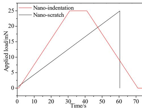
**Figure 3.** Loading-unloading curves of nano-indentation and nano-scratching.
