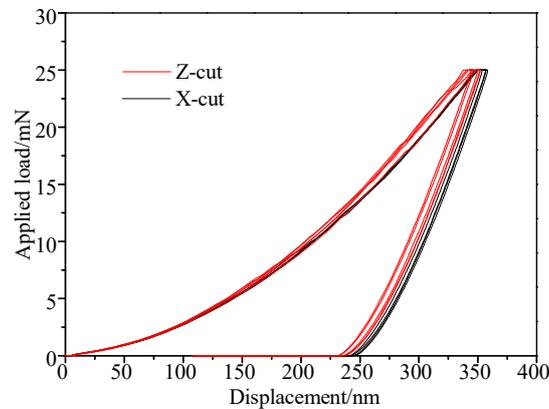
Figure 5. Applied load-displacement curves of Nano-indentation tests.
