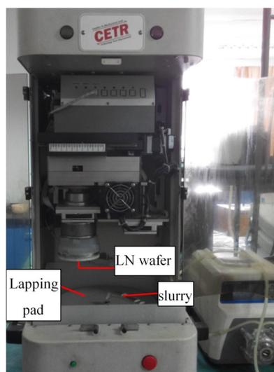
**Figure 4.** Fixed-abrasive lapping tests with CP-4 test system.
