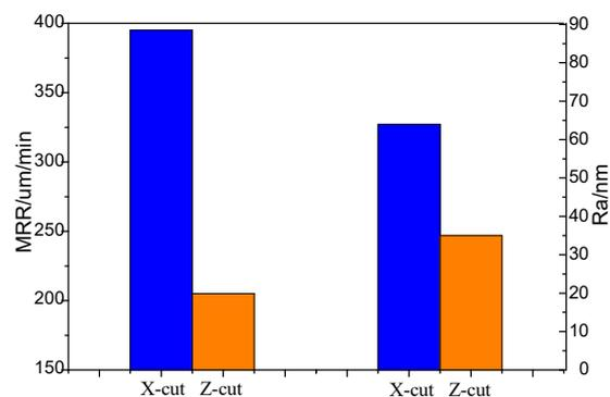
Figure 12. MRR and Ra of Z-cut and X-cut.
