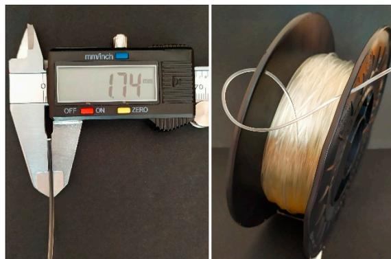
**Figure 2.** View of obtained TPU\_F filament.
