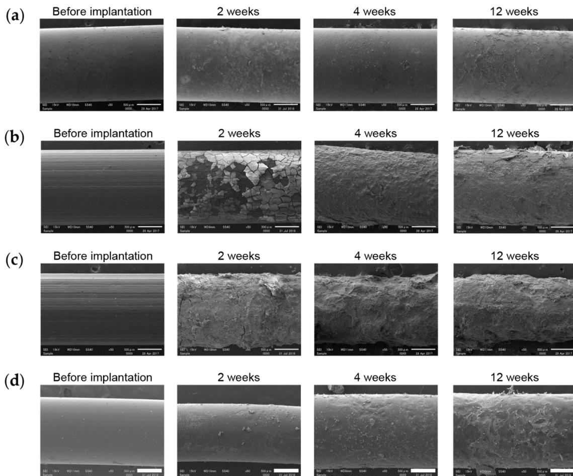
**Figure 10.** Representative scanning electron microscopy (SEM) images of the implant surface removed during biomechanical push-out testing. (a) TiA, (b) MgA, (c) Mg and (d) PLA implants. SEM image, 100× magnification. Scale bars at lower right, 500 µm.
