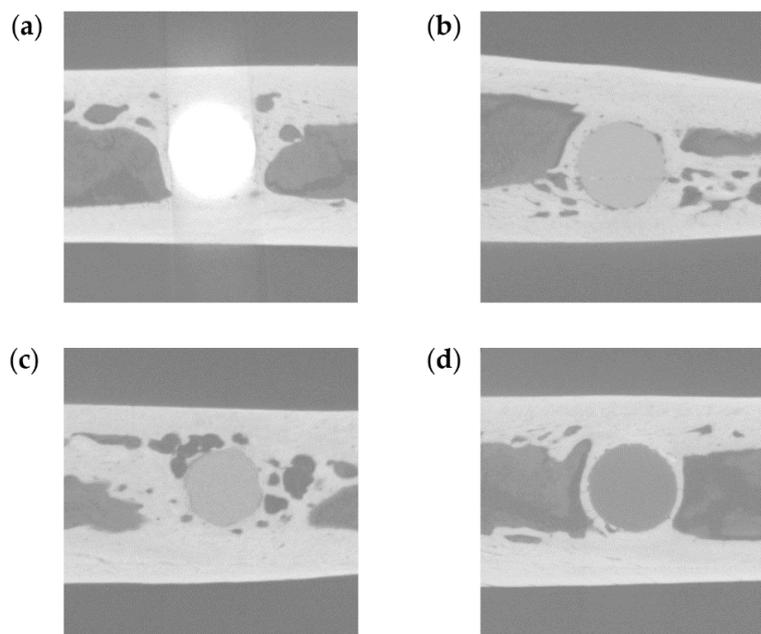
**Figure 3.** Representative micro-computed tomography (CT) images. (a) TiA, (b) MgA, (c) Mg, and (d) PLA implants.
