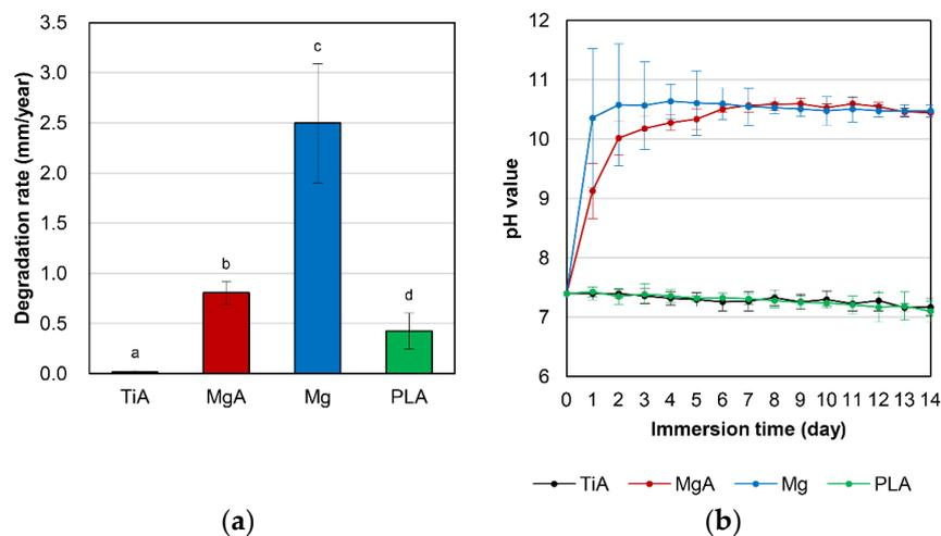
**Figure 6.** (a) Degradation rate (mm/year) and (b) pH change in the solution when samples were immersed in simulated body fluid (SBF) for 14 days. Identical letters indicate no significant difference ( $p < 0.05$ , Tukey's test).
