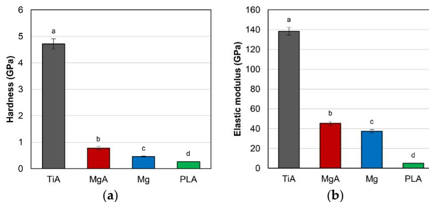
**Figure 5.** (a) Hardness (GPa) and (b) elastic modulus (GPa) of the implants as determined by nanoindentation testing. Identical letters indicate no significant difference ( $p < 0.05$ , Tukey's test).
