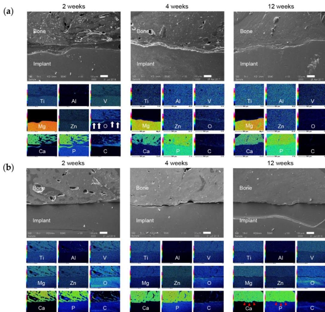
**Figure 12.** Representative SEM images and energy dispersive X-ray spectroscopy (EDX) elemental mapping of the bone-implant interface. (a) Mg and (b) PLA implants. SEM image, 100× magnification. Scale bars at lower right, 100 μm. EDX elemental mapping corresponds to the SEM image. White arrows indicate the oxide layer of the Mg implant, red arrowheads indicate new bone formation (existence of Ca and P).
