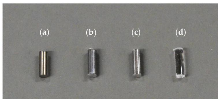
**Figure 1.** Photograph of prepared implant samples. (a) titanium alloy (TiA): American Society for Testing and Materials (ASTM) B348 Gr5 (Ti-6Al-4V) titanium alloy, (b) magnesium alloy (MgA) AZ31 magnesium alloy, (c) Mg: pure magnesium, (d) poly-L-lactic acid (PLA): ISO 13,485 compliant medical poly-L-lactic acid. Each material was processed into a cylindrical shape with a diameter of 1.6 mm and a length of 4.0 mm.
