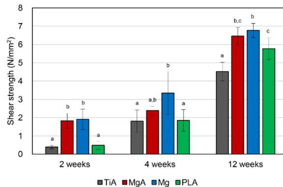
**Figure 9.** Shear strength of the bone-implant interface as determined using biomechanical push-out testing ( $\text{N/mm}^2$ ). Significantly higher shear strength was observed in the MgA group compared to the TiA group. Identical letters indicate no significant difference ( $p < 0.05$ , Tukey's test).
