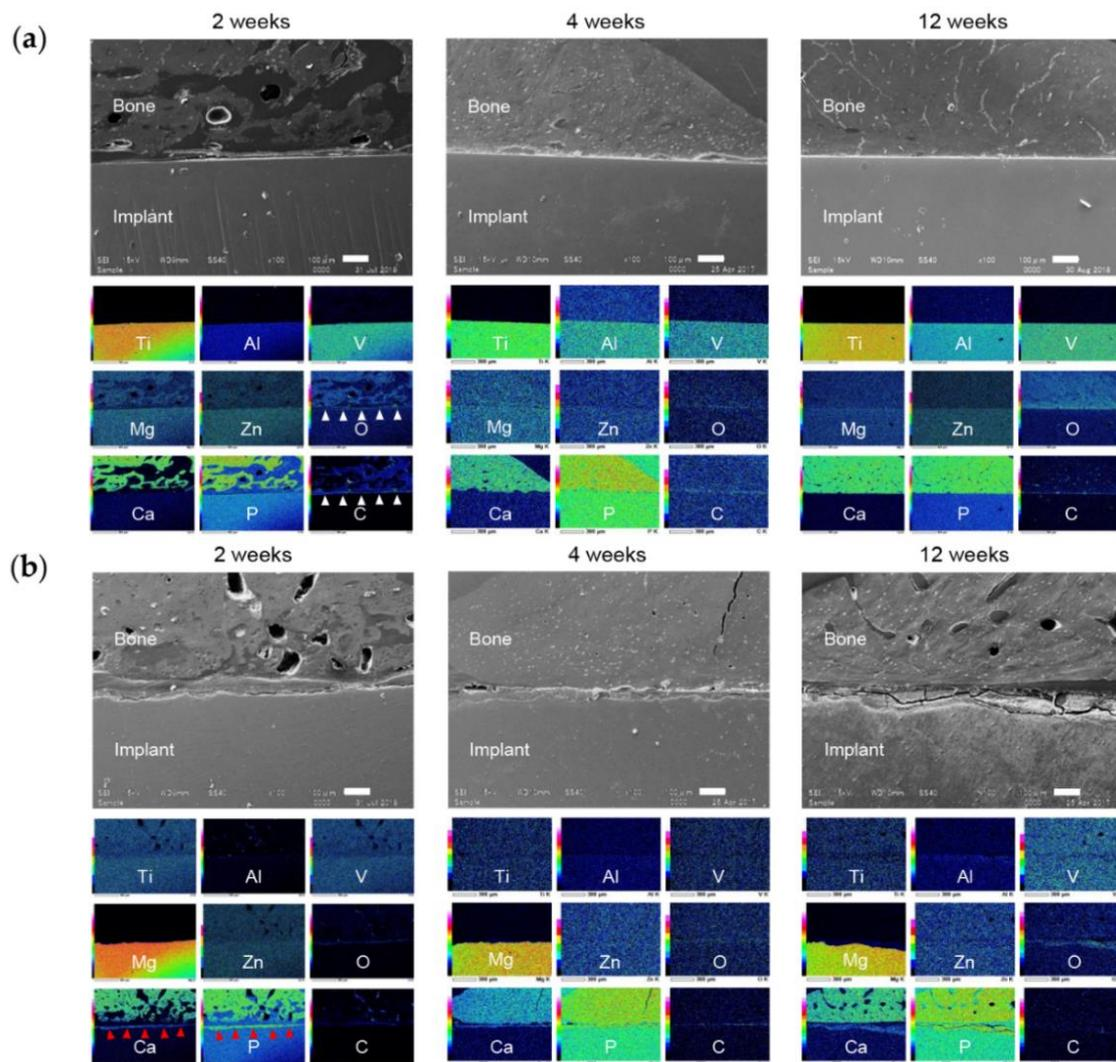
**Figure 11.** Representative SEM images and energy dispersive X-ray spectroscopy (EDX) elemental mapping of the bone-implant interface. (a) TiA and (b) MgA implants. SEM image, 100× magnification. Scale bars at lower right, 100 μm. EDX elemental mapping corresponds to the SEM image. White arrowheads indicate fibrous tissue (existence of O and C), red arrowheads indicate new bone formation (existence of Ca and P).
