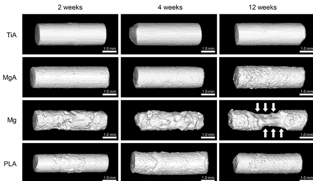
**Figure 7.** Three-dimensional reconstructions of implants based on the micro-computed tomography (CT) data. No changes were observed in the TiA group. Absorption from the surface layer, which increased over time, was observed in the MgA, Mg and PLA groups. Marked absorption at the portion in contact with the bone marrow (white arrow) at 12 weeks was observed in the Mg group.
