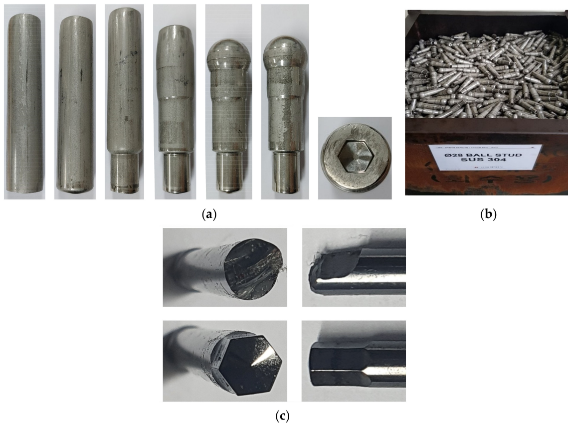
Figure 14. Experiments of SUS304 ball-stud forging: (a) experiments; (b) a lot of manufacture; (c) die failures (upper: fatigue fracture, lower: wear).
