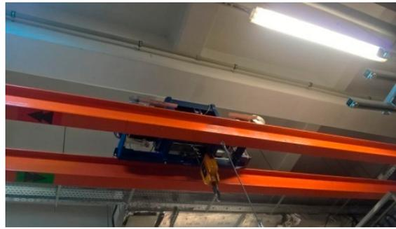
**Figure 2.** The tested double-girder overhead traveling crane with a trolley and a hoist.
