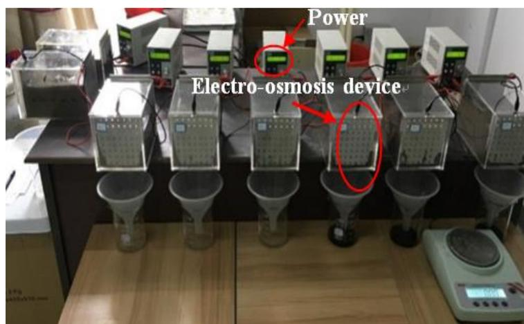
Figure 2. Setup of electro-osmosis test.
