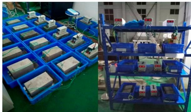
**Figure 2.** Experiment of bidirectional electromigration (BIEM).
