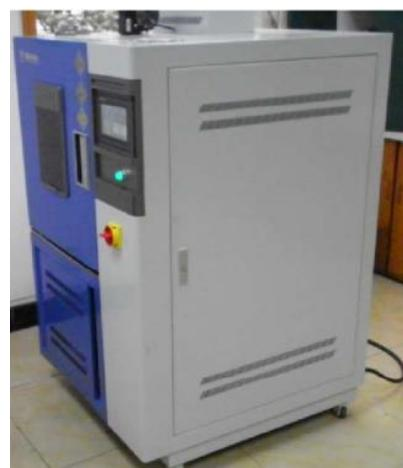
**Figure 1.** RG-80 asphalt aging test chamber.
