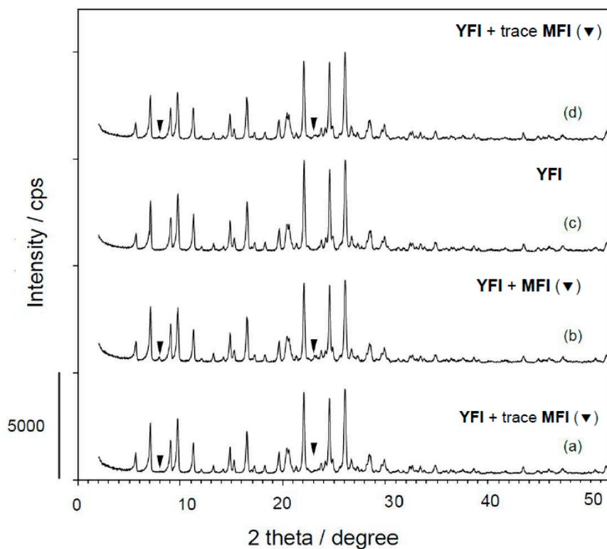
**Figure S3.** Powder X-ray diffraction patterns obtained from the (a) deAl-YFI-A(51), (b) deAl-YFI-B(57), (c) deAl-YFI-C(55), and (d) deAl-YFI-D(63).
