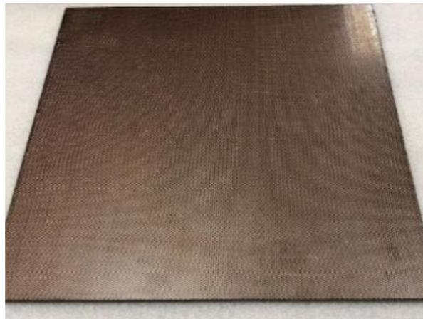
Figure 4. Test panel with ECF (L\_ECF). Dimensions: 300 mm × 300 mm.
