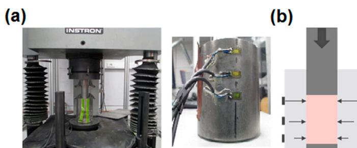
**Figure 2.** (a) Pressing machine used for formation of green bodies, location of radial stress measurements; (b) schematic representation of cylindrical green body with pressure sensor locations.
