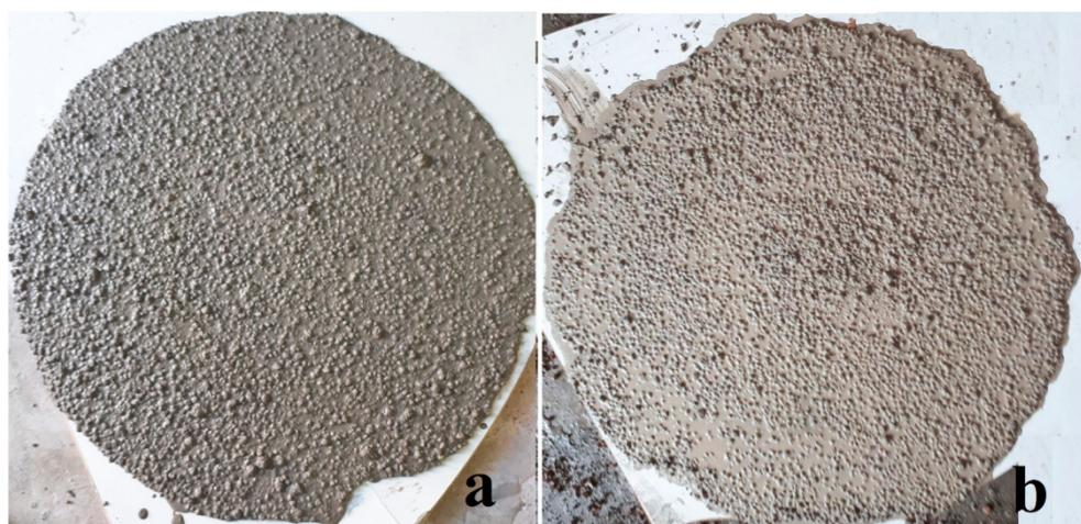
**Figure 5.** Appearance of the LWCs after the flow test: (a) Mix with 3 wt.% NS and (b) mix without NS, reprinted with permission from ref. [23] Copyright 2018, Elsevier.
