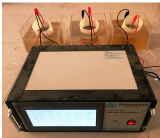
**Figure 15.** Test device for the rapid chloride migration (RCM) method, reprinted with permission from ref. [117].
