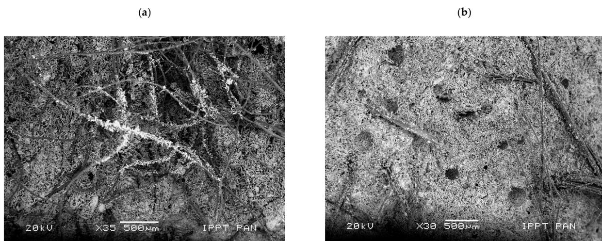
**Figure 9.** Microphotograph of the analysed fresh split surface of gypsum-based composites: (a) with sheep wool fibres and (b) with hemp fibres (scanning electron microscope, scale bar = 500  $\mu\text{m}$ ).
