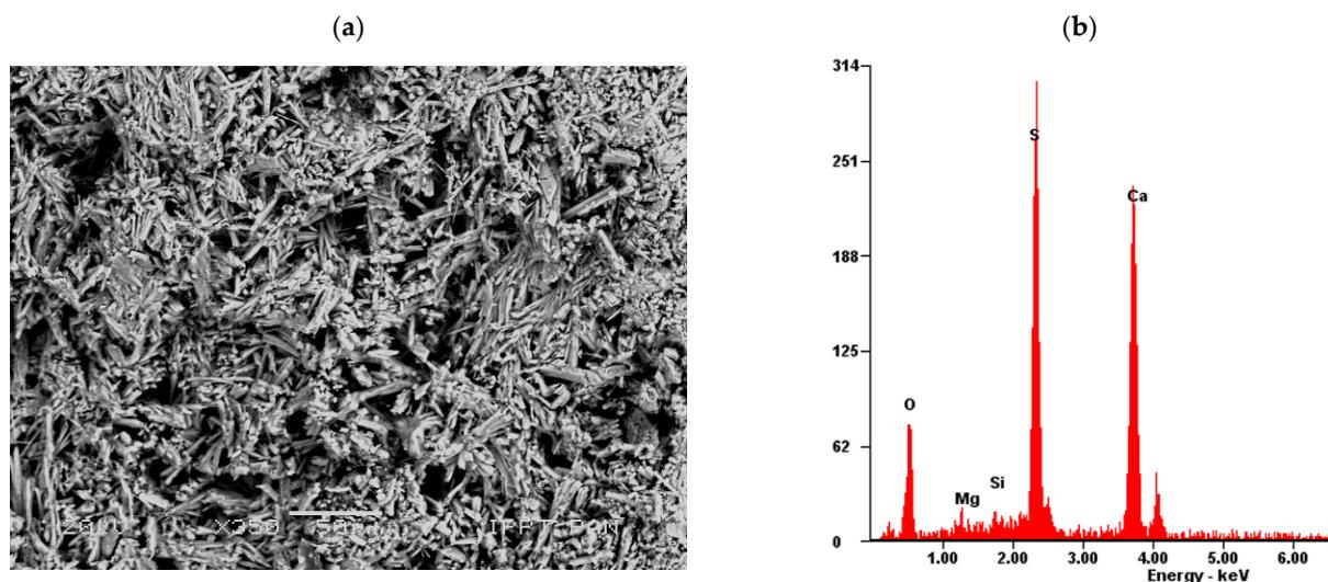
**Figure 8.** The analysed fresh split surface of gypsum paste: (a) SEM microphotograph and (b) EDS analysis in the reference specimen without fibres—Series ref; S-Sulphur, Ca-Calcium, Mg-Magnesium, Si-Silicon (scanning electron microscope, scale bar = 50  $\mu\text{m}$ ).
