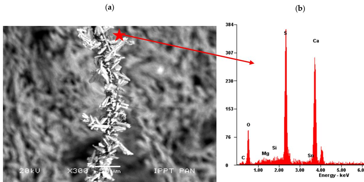
**Figure 11.** A single sheep wool fibre completely overgrown with gypsum crystals: (a) SEM microphotograph and (b) EDS analysis: S-Sulphur, Ca-Calcium, Si-Silicon, Mg-Magnesium, O-Oxygen (scanning electron microscope, scale bar = 50 µm).
