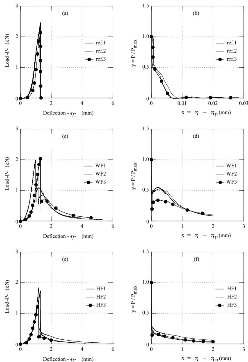
**Figure 6.**  $\eta$ - $P$  and  $x$ - $y$  curves experimentally obtained with the flexural tests; reference specimens A—(a,b), specimens with sheep wool fibres B—(c,d), specimens with hemp fibres C—(e,f).
