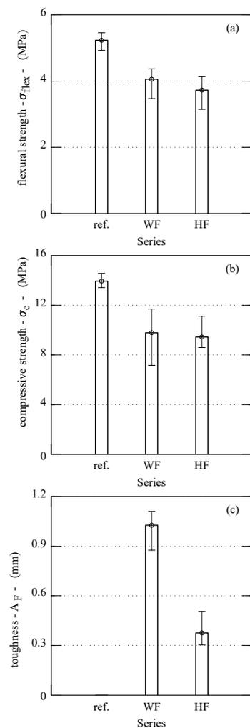
**Figure 7.** Average values of: (a) flexural strength, (b) compressive strength, and (c) flexural toughness of gypsum composites.
