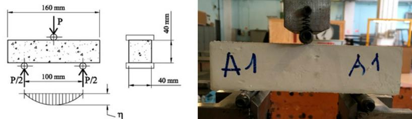
Figure 3. Three-point bending test on gypsum composites.
