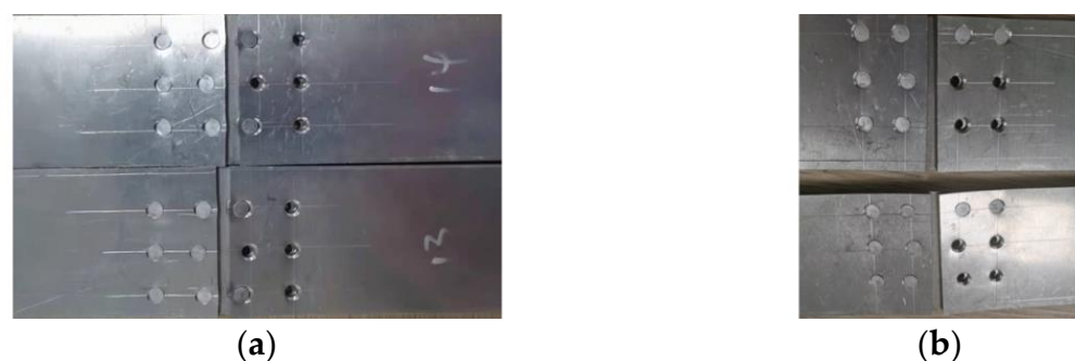
Figure 19. Part of the connector rivets fall off: (a) increase the rivet row spacing at both ends of the inner side; (b) decrease the rivet row spacing at both ends of the inner side.
